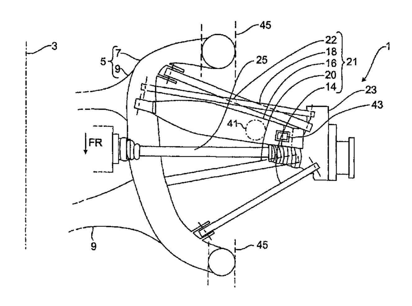
respect to the spring link is of softer design in the transverse direction of the vehicle than the rear pair of links. As a result, a change in the toe-in at the rear wheel takes place under exertion of a lateral force or a longitudinal force.
