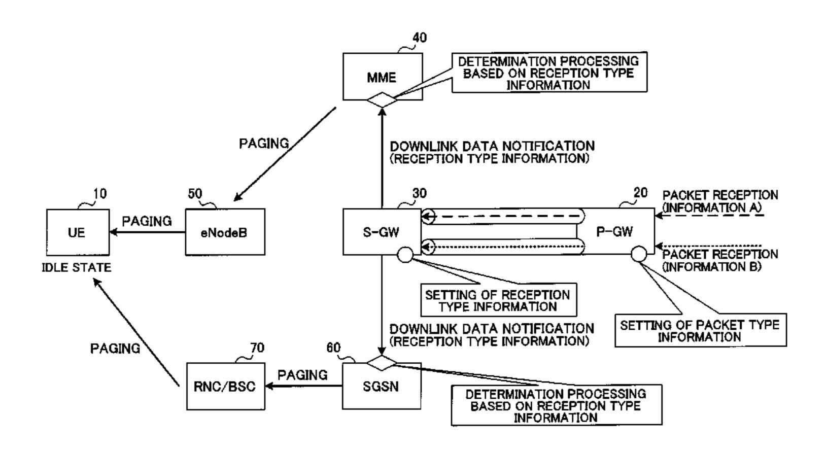
and SGSN (60), determining whether or not to page the UE (10) based on the reception type information included in the "Downlink Data Notification" from the S-GW (30).
