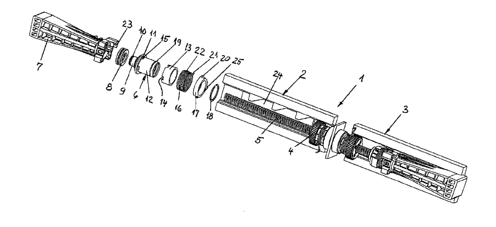
spindle, moved in the axial direction of the threaded spindle. The linear drive has a lifting element for adjusting the moveable furniture parts, the lifting element being driven by axial movement of the spindle nut. Simple design, easy assembly and operation, and robust mounting of the driving parts are achieved.
