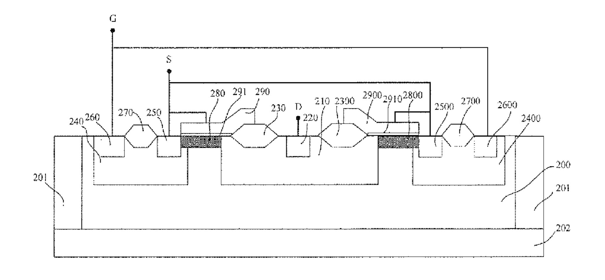
source electrode electrically is led out from a connection of the field electrode plate and the second conductivity type source heavily doped region; and a gate electrode electrically is led out from the first conductivity type gate heavily doped region. The transistor has a high breakdown voltage and easy to be integrated.
