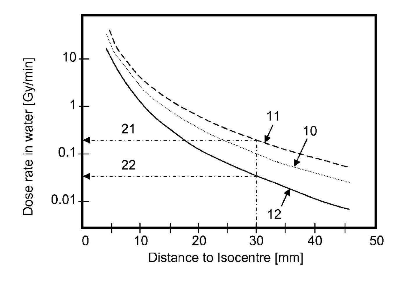
X-ray radiation, with defined second radiation characteristics, in particular with a predetermined second radiation dose rate curve (12).
