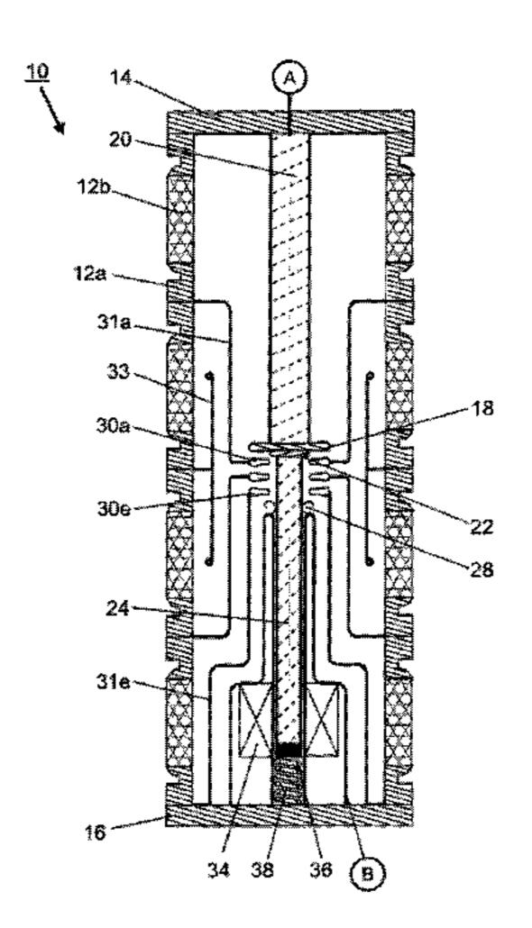
breaker according to the invention can be advantageously used in vehicles and in ultra-high-voltage AC and HVDC (high-voltage direct current) transmission systems and causes arcs to be extinguished as early as possible during the switching process.
