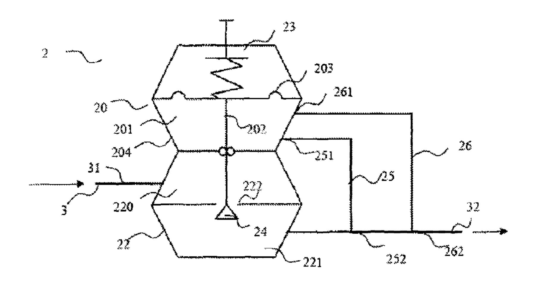
device are arranged on the chamber. The drive device and the valve including such a drive device can exhaust air entering the chamber along with the working medium out of the chamber by the vents on the chamber thereby optimizing the performance of the drive device and the valve and helping to keep the valve operating in a stable manner.
