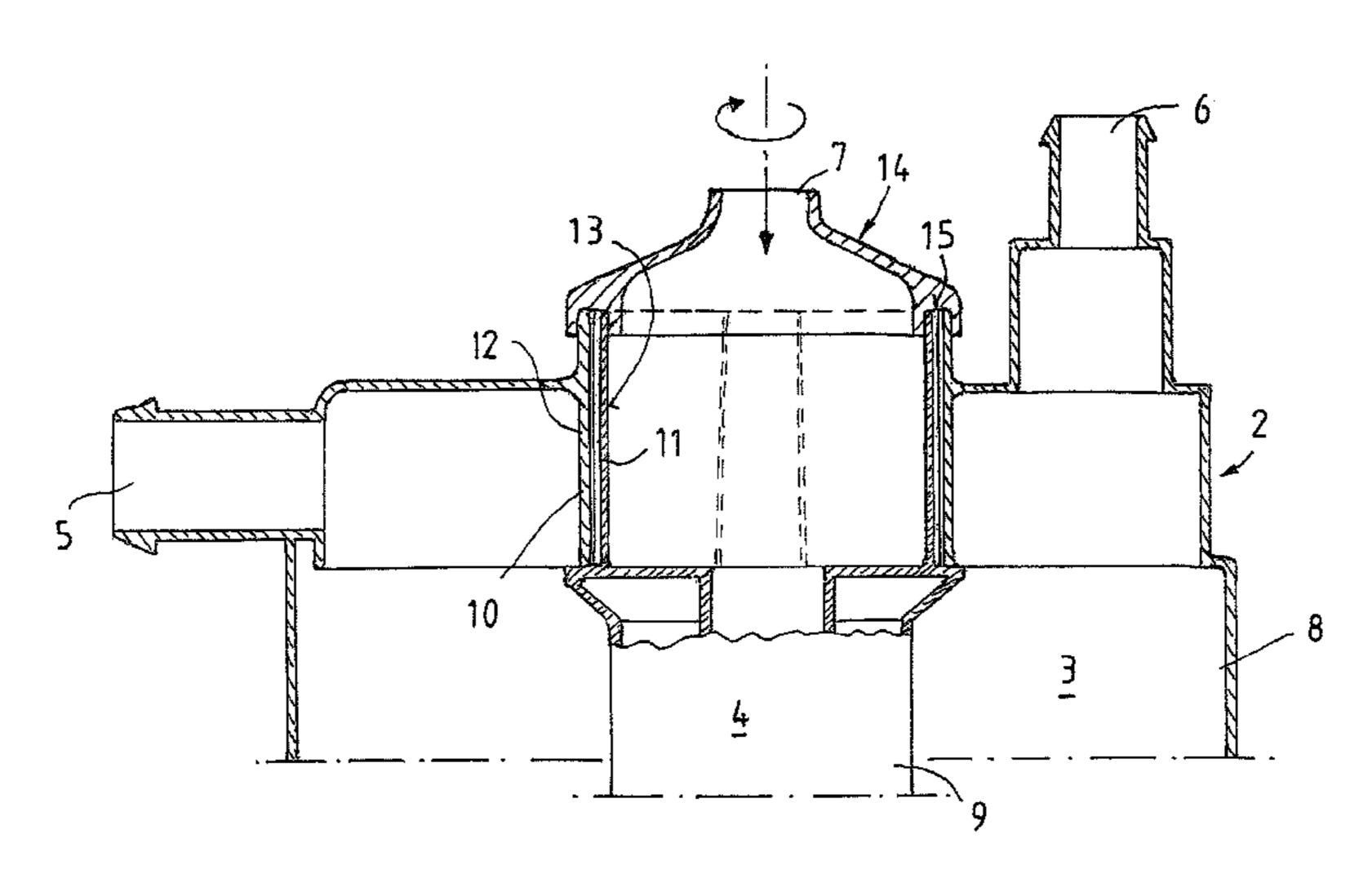
wall of the outer housing member (8) and wherein the inner housing member (9) and the outer housing member (8) are sealed against each other by means of a closure cap (14).
