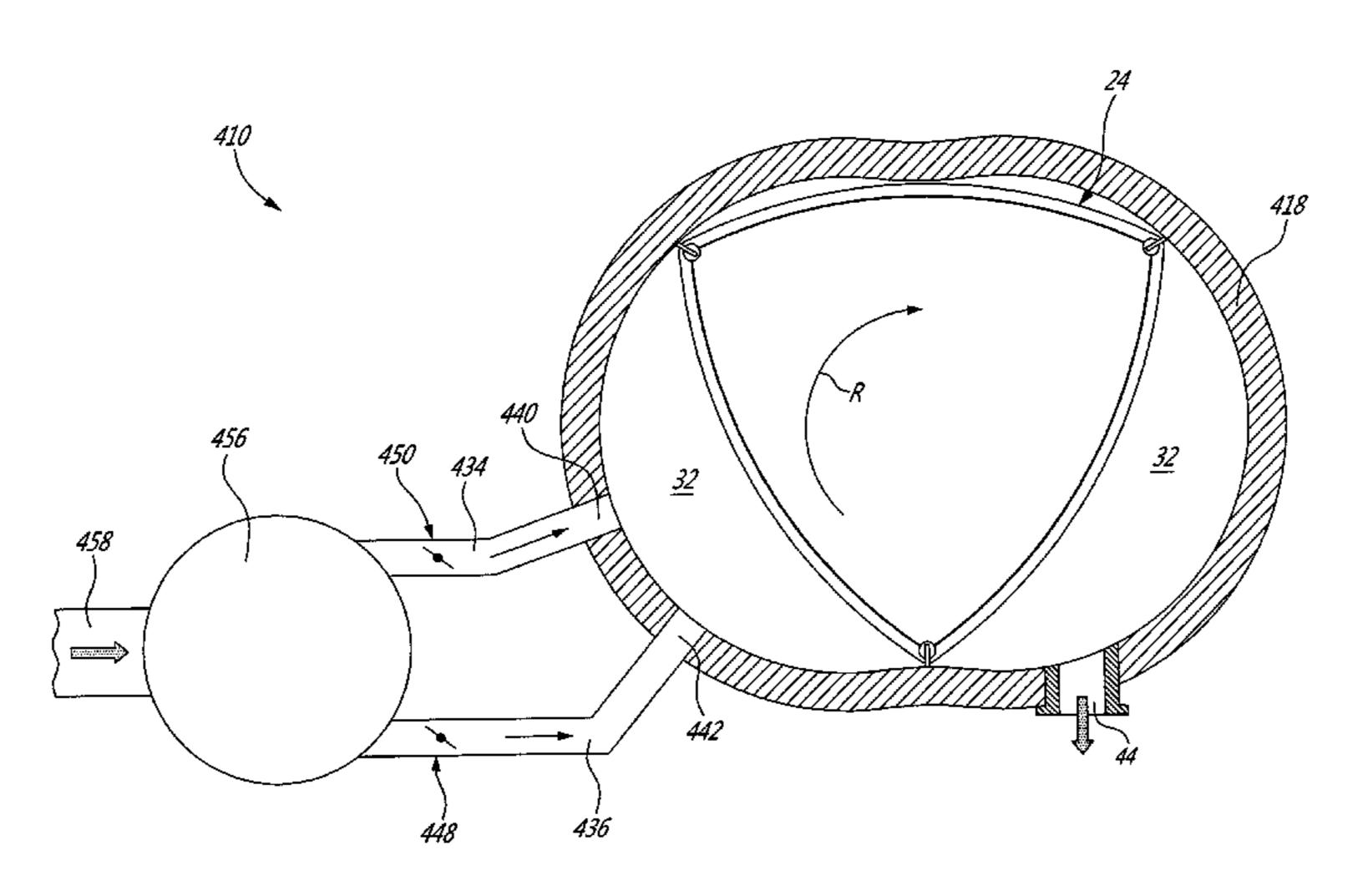
inlet port, the secondary inlet port being located such as to be in communication with the exhaust port throughout portions of the revolution of the engine to purge exhaust gases of the engine.
