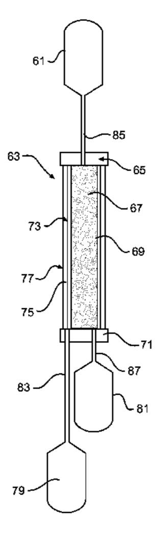
the outer wall and the membrane, wherein the plasma which permeates through the membrane enters the outer chamber and exits the filter device via the first outlet; whereby the blood which has been depleted of oxygen and/or carbon dioxide, leukocytes and plasma exists and filter device via the second outlet.
