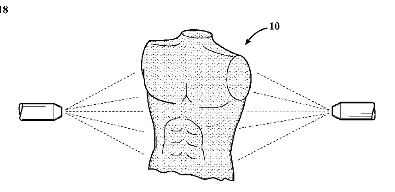
an elastomeric polyurethane composition upon the rigid polyurethane foam shell after demolding to form the elastomeric polyurethane layer.
