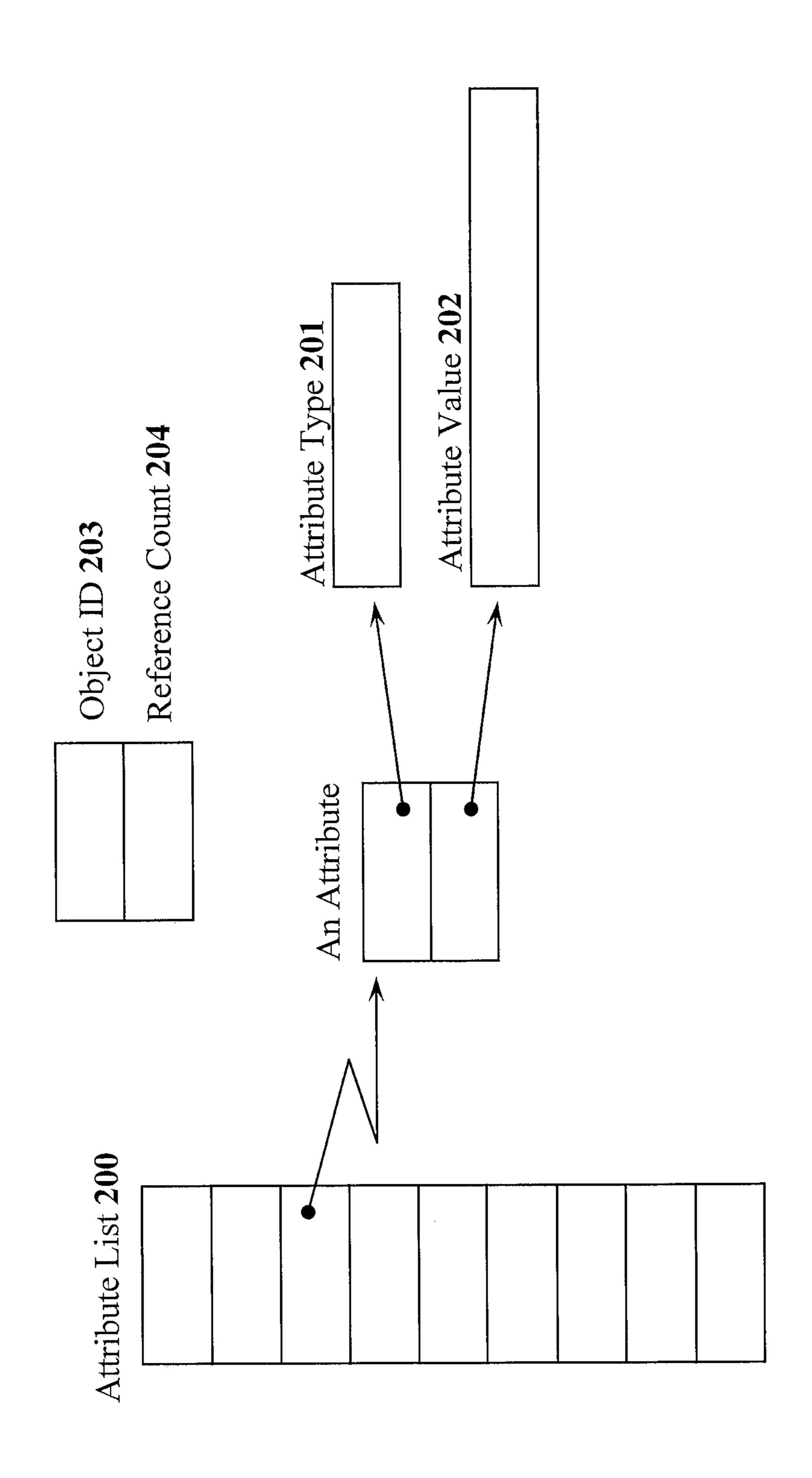
Fig. 2: Structure of a Viewing Object
