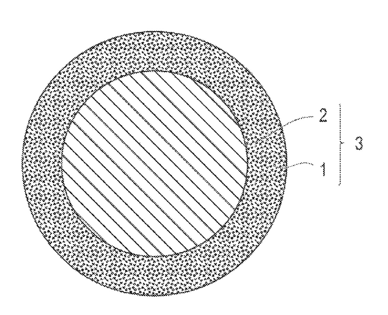
primary particles (D1) and the standard deviation ( $\sigma$ ) of the average particle diameter of the primary particles (D1) meet the relationship of D1/ $\sigma^2 \ge 24$ .
