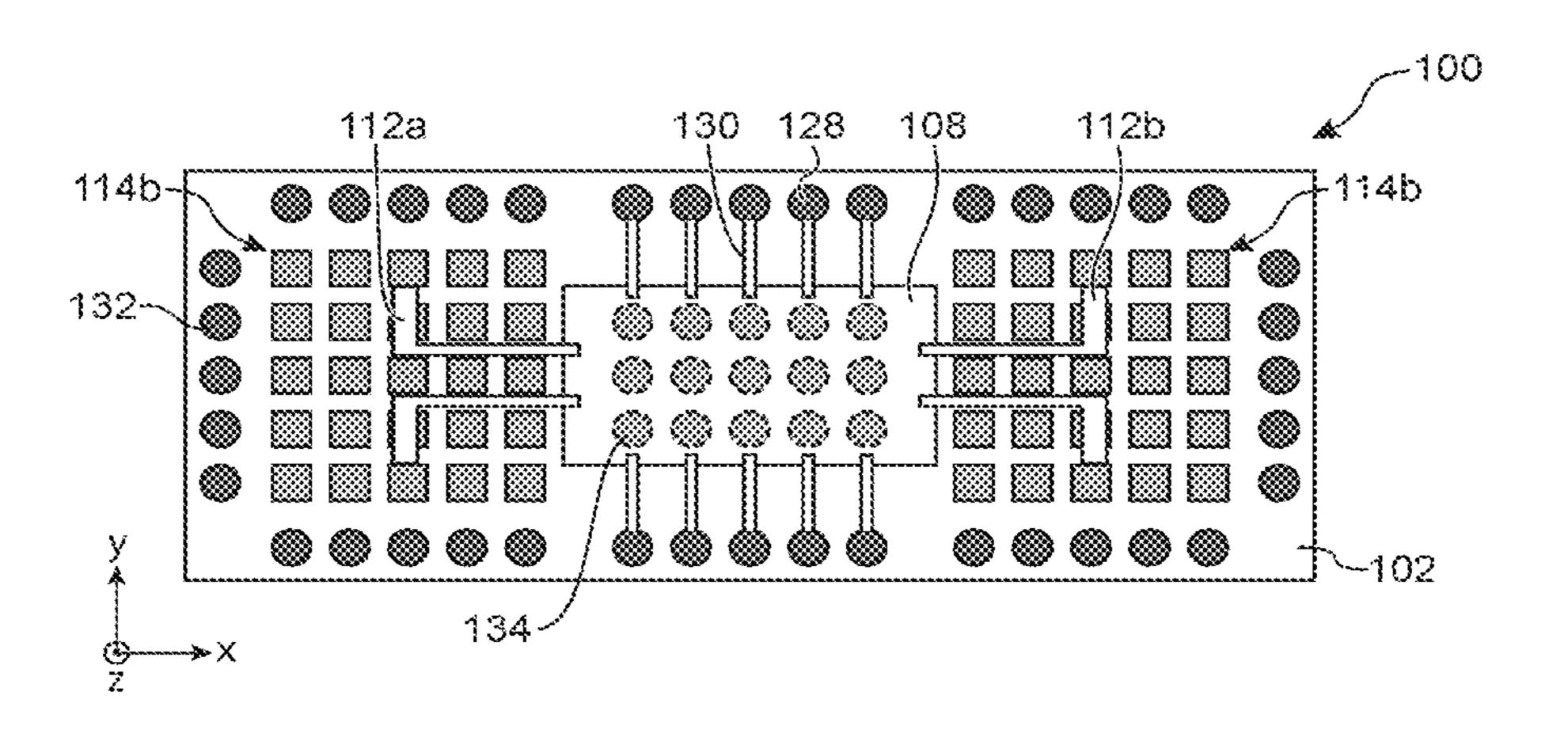
ing a first periodic structure and arranged on the first face of the substrate opposite the first antenna; a first electrically conducting ground plane arranged at least partially opposite the first antenna.
