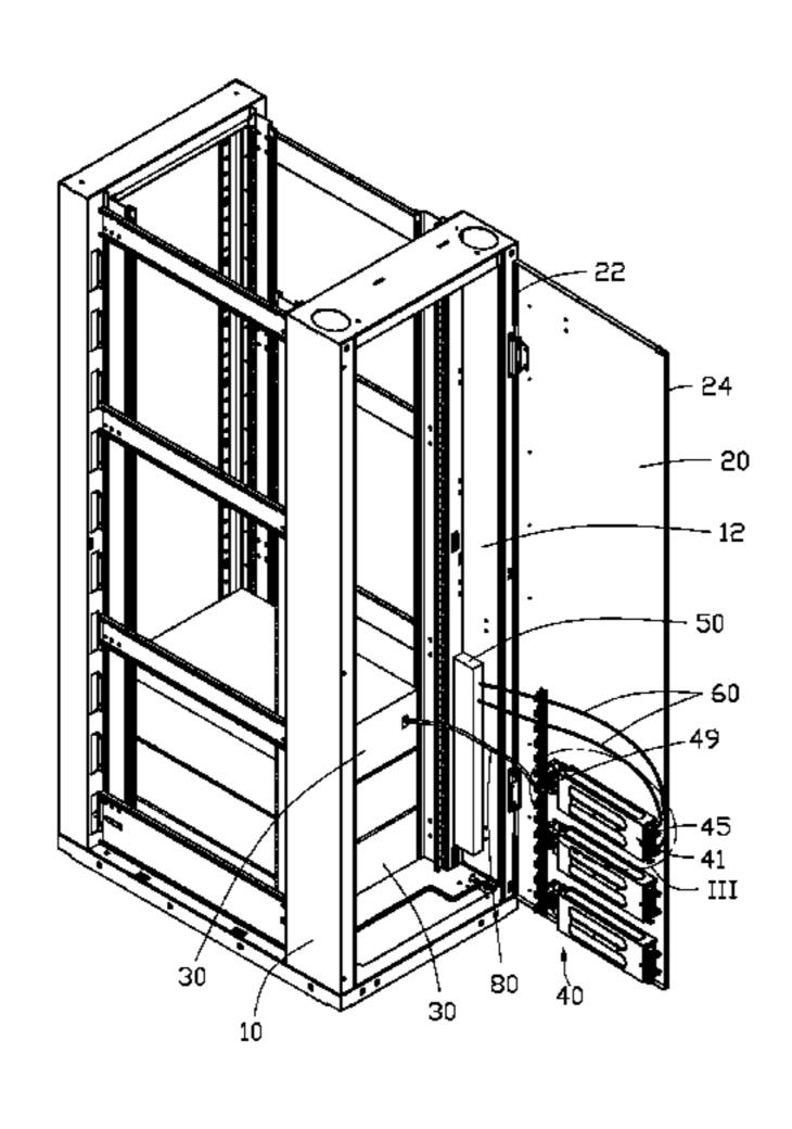
ity of cables, the power supply units being detachable and replaceable in spite of minimal physical access through the partly-closed door.
