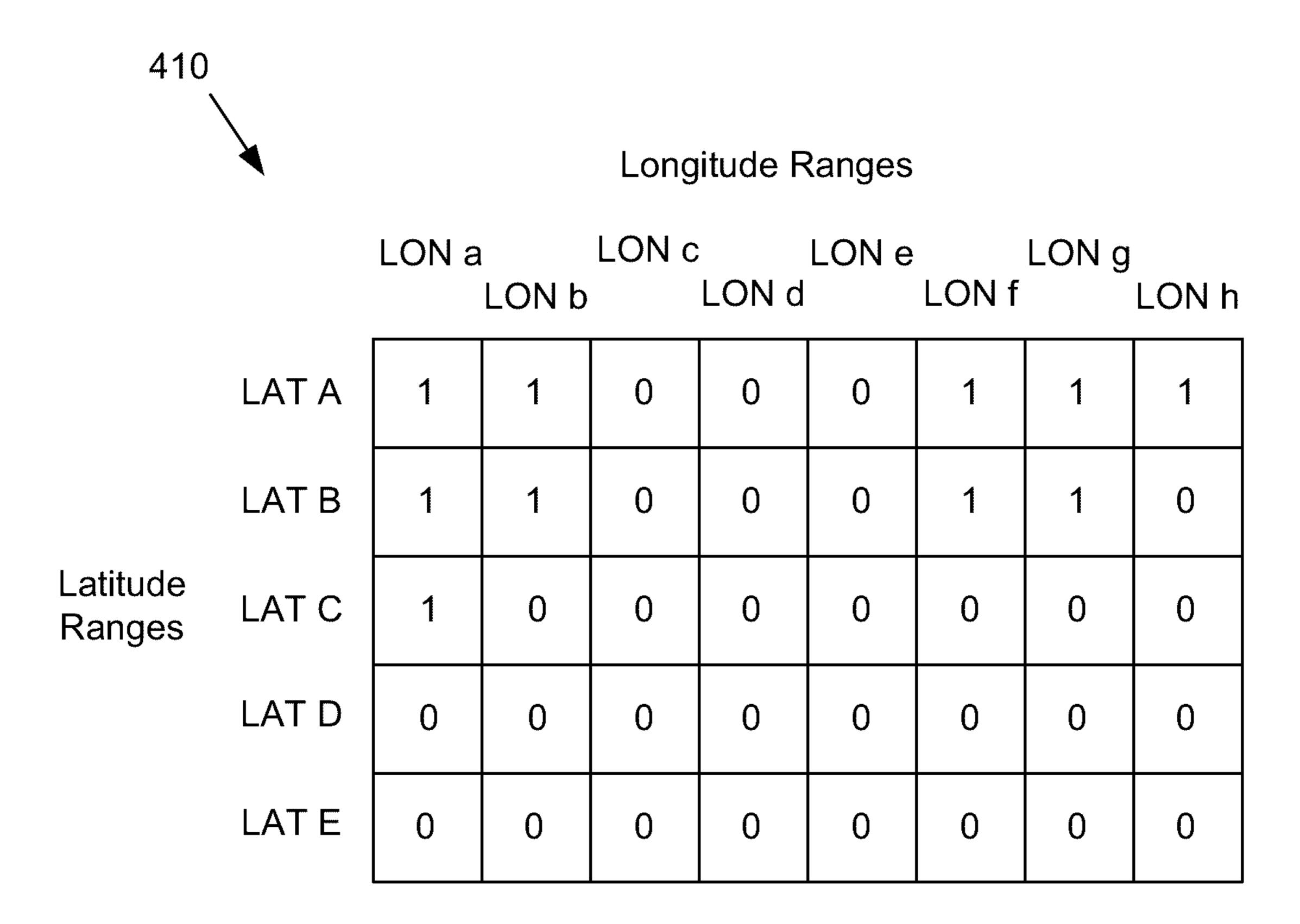
Tile Set Representation Of An Altitude Difference That Is Equal Or Greater Than An Altitude Threshold
