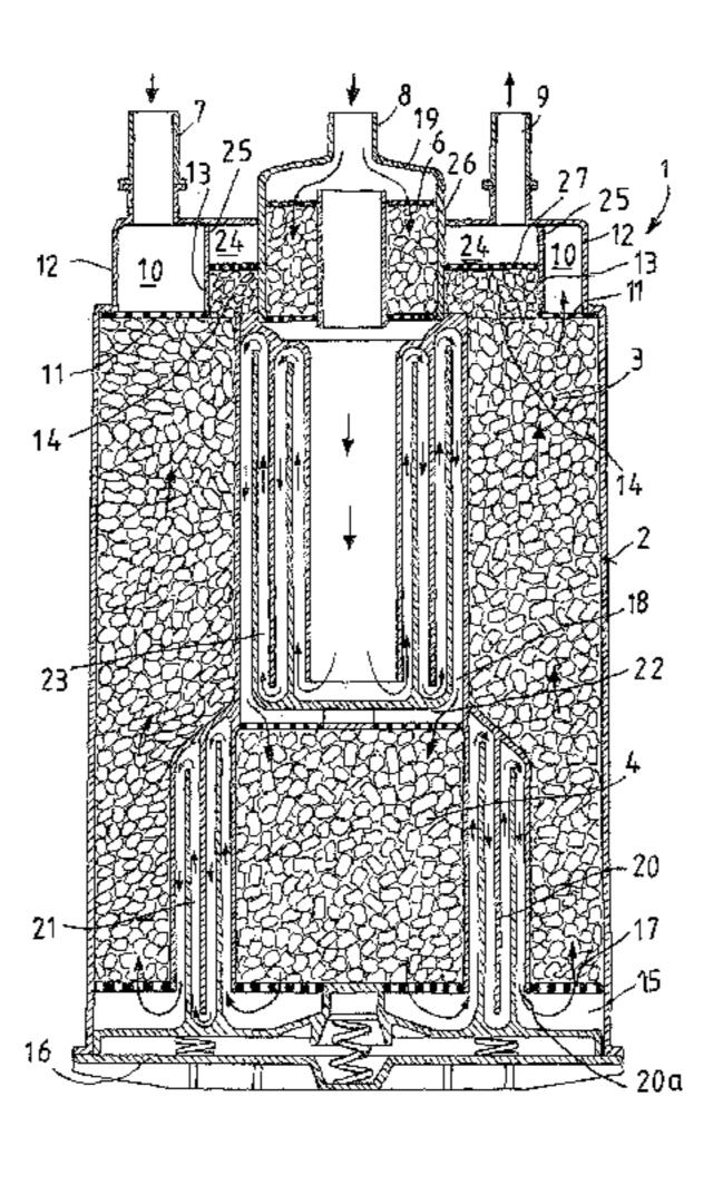
adsorbent material. Said first fuel vapor distribution chamber is arranged upstream said purge buffer zone (14) and communicates with said fuel vapor inlet port (7). Said second fuel vapor distribution chamber (24) is arranged downstream said purge buffer zone and communicates with said purge port (9).
