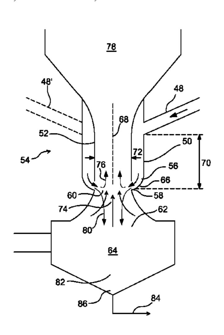
section. A reagent in the reaction chamber converts pollutant compounds in the gas stream to reaction products. A discharge channel in flow connection with the reaction chamber discharges gas and particles including the reaction products from the reaction chamber. A particle separator separates particles from the gas. A return channel recycles a portion of the particles to the reaction chamber.
