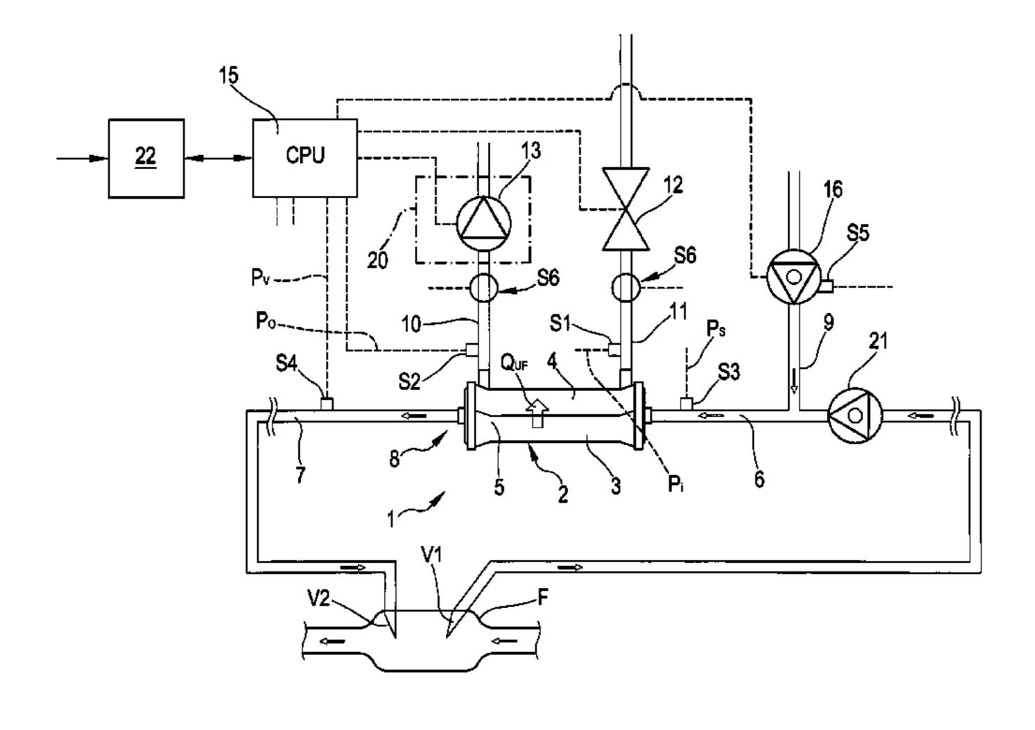
to: command the regulating device (20) by setting a first increase (STMP<sub>1</sub>), determine a value of a control parameter ( $\phi_1$ ) corresponding to the first increase, compare the value of the control parameter ( $\phi_1$ ) with a reference value ( $\phi_{ref}$ ) and, if the value of the control parameter is greater than the reference value, command the regulating device (20) by setting a second increase (STMP<sub>2</sub>) which is greater than the first increase (STMP<sub>1</sub>).
