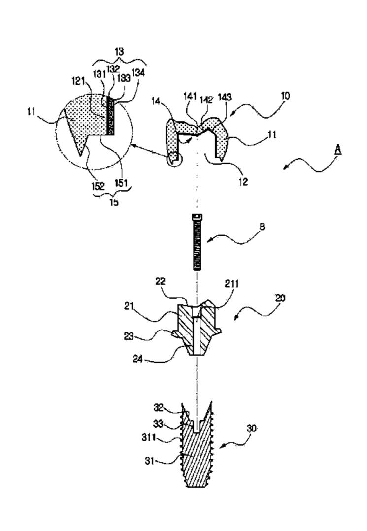
detachment and smooth repair and correction. The crown is made using milling, thus reducing errors to ensure good fitness and passivity.
