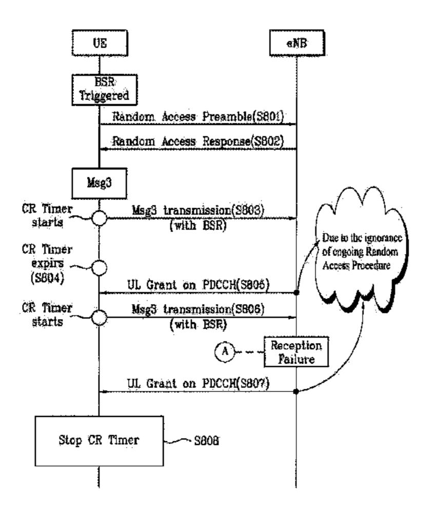
Msg3 buffer when receiving the UL Grant signal on the specific message and the specific message is the random access response message.
