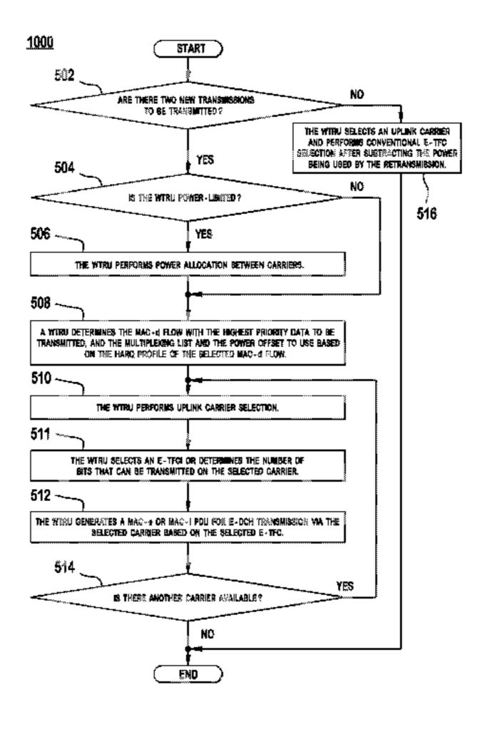
transmission via the selected carrier based on the selected E-TFC.
