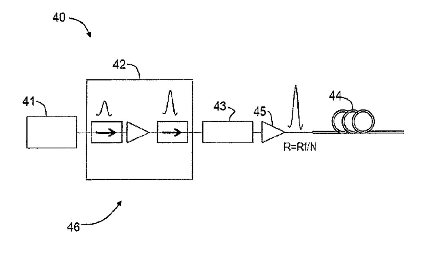
comprises a second gating device provided after the non-linear optical element.
