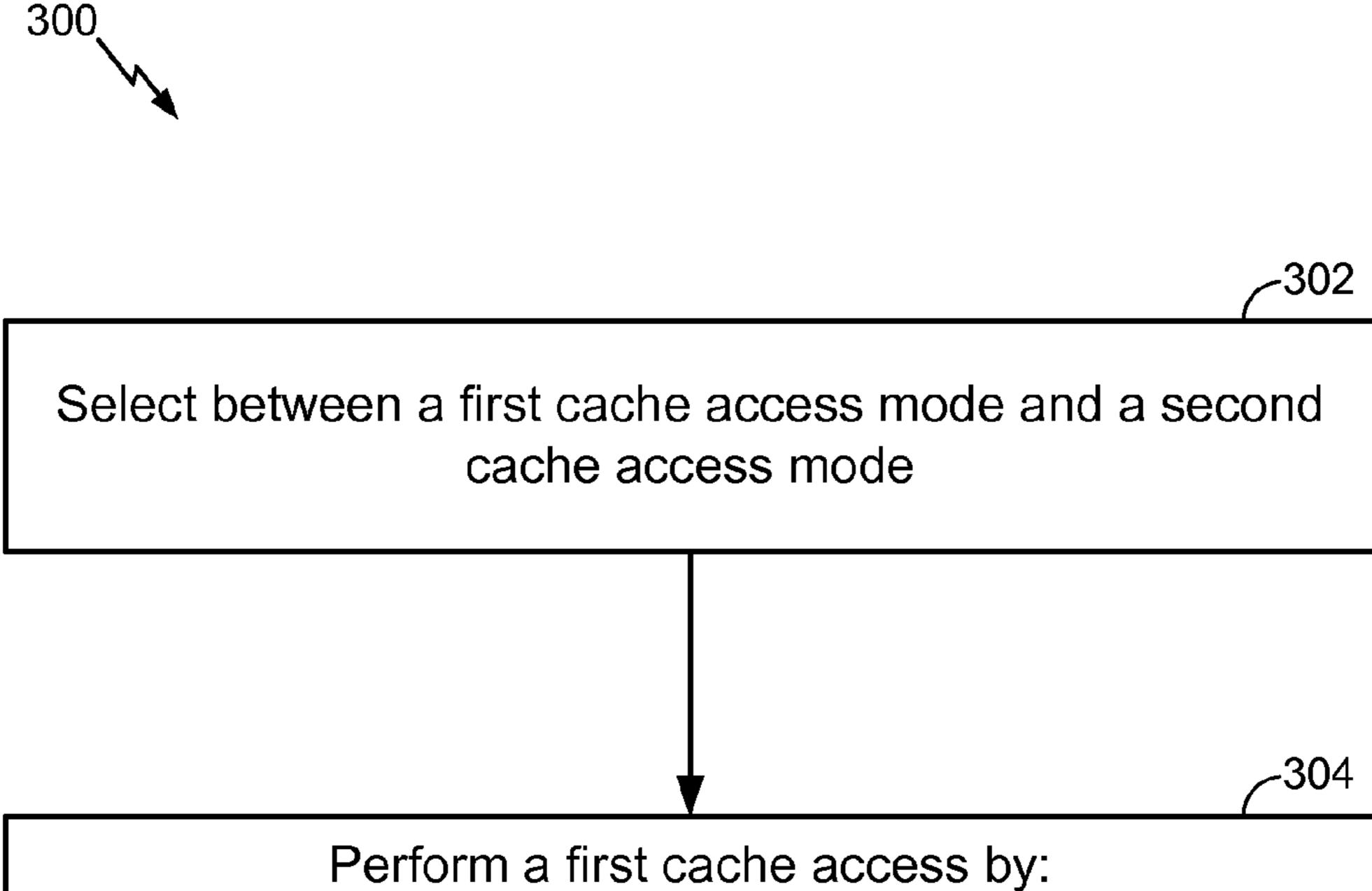
when the first cache access mode is selected, perform a tag access and perform a data array access after performing the tag access; when the second cache access mode is selected, perform the tag access in parallel with the data array access
