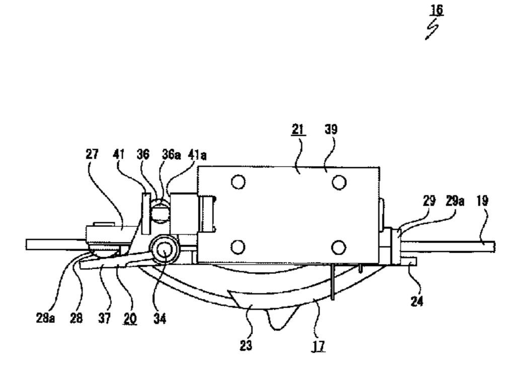
contact portion (37) in accordance with a displacement of the link member (20). A surface (28a) of the projection (28) is formed as a curved surface.
