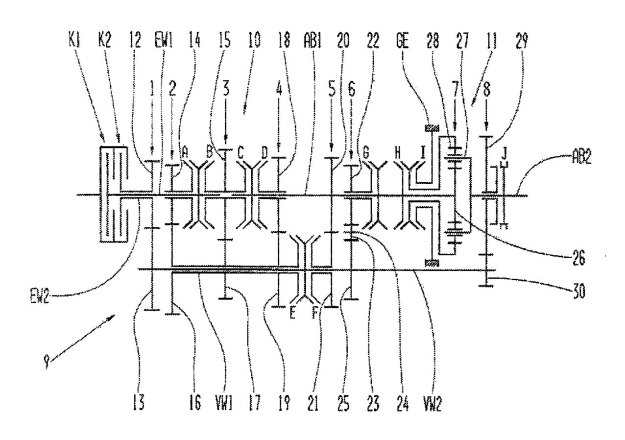
second countershaft can be connected via a shifting element to the group transmission drive output.
