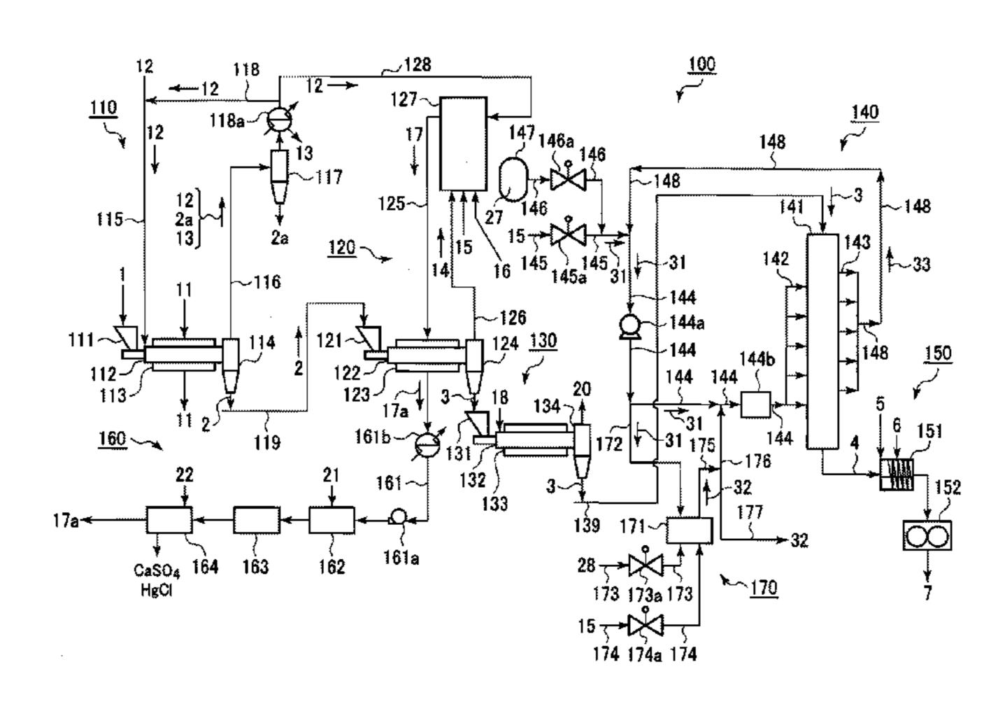
means (142-144, 144a, 145, 145a, 146, 146a, 147, 148) that feeds processing gas to the interior of the device main body (141); a processing gas circulation means (148) that circulates used processing gas (33) used in the device main body (141) to the processing gas feed means; and a carbon monoxide processing device (170) that adjusts the carbon monoxide concentration in the processing gas in a manner so as to reduce the carbon monoxide concentration in the processing gas.
