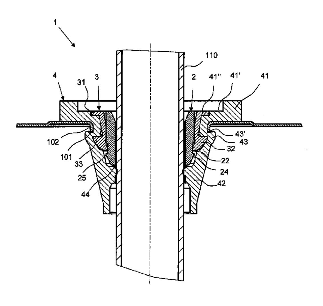
hooks (33) of the spreading ring (3) are turned outward and engage in the bulge (43), whereby a circumferential projection is pressed in the direction of an underside of the ring flange (41).
