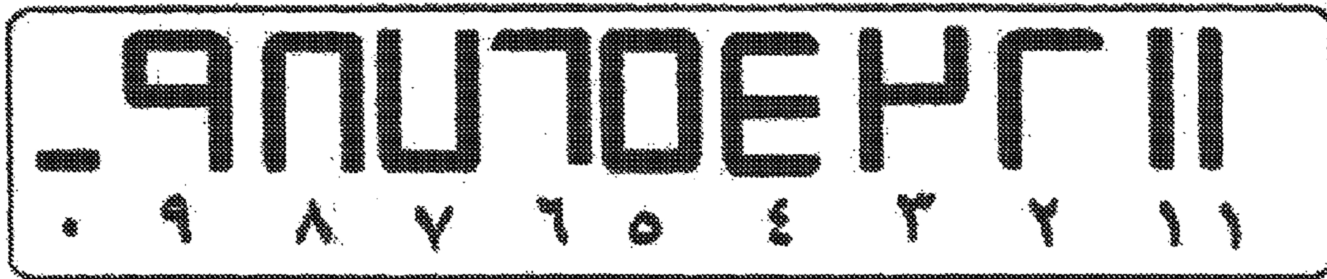
Referenced Method and System: Seven Segment Indian Numeral Character Inverse Encoding
