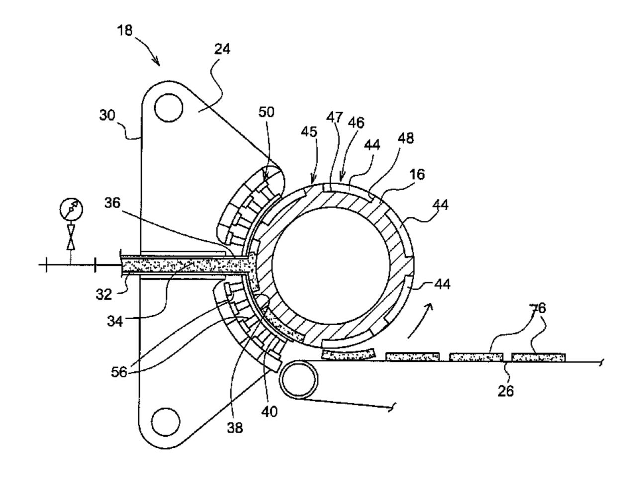
dispensing mouth (36) with respect to each other. A control unit controls the pump on the basis of the position-determining device during the movement of the mold cavity (44) opening and the dispensing mouth (36) with respect to each other.
