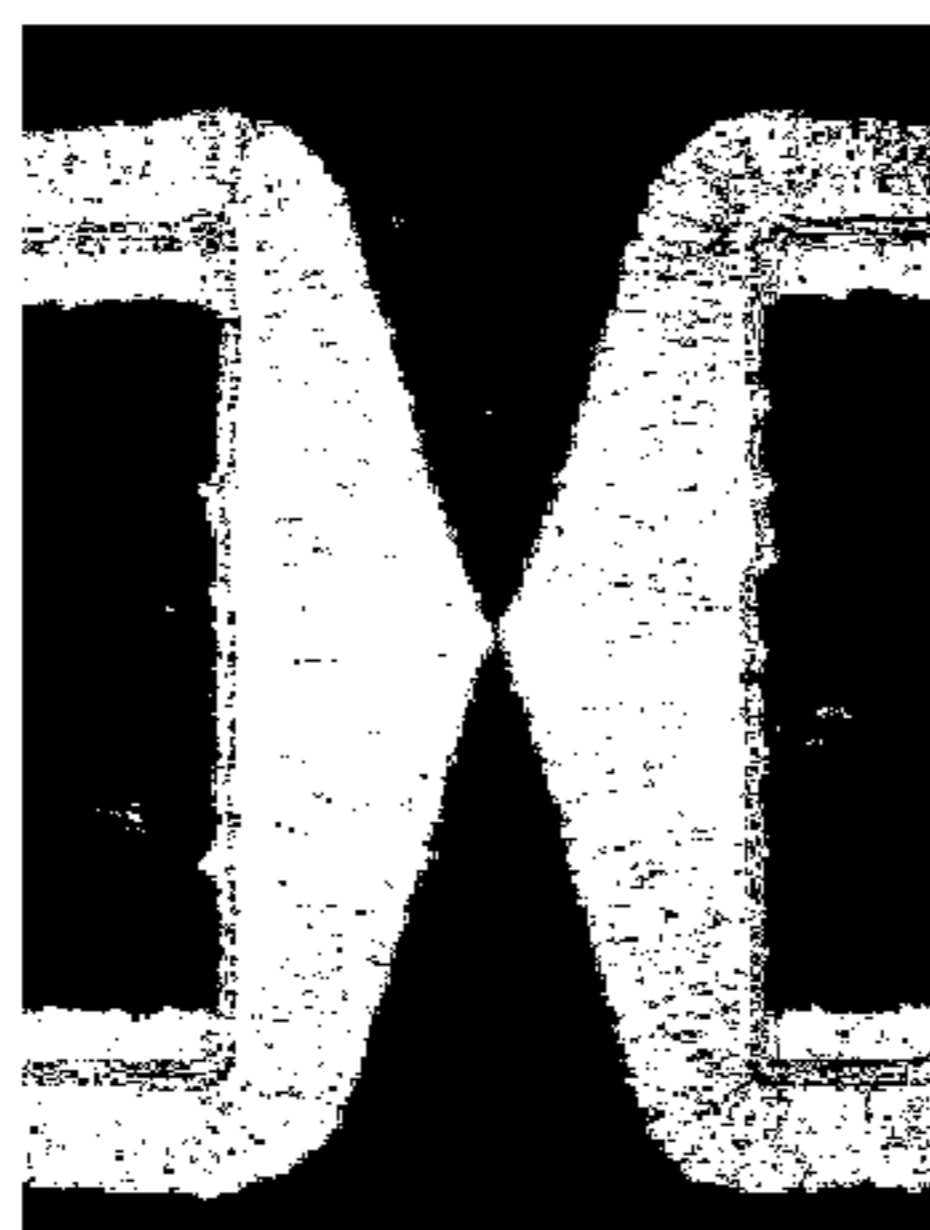
Formation of a narrow part due to preferred copper-plating in the center of a through-hole in a printed circuit board.
