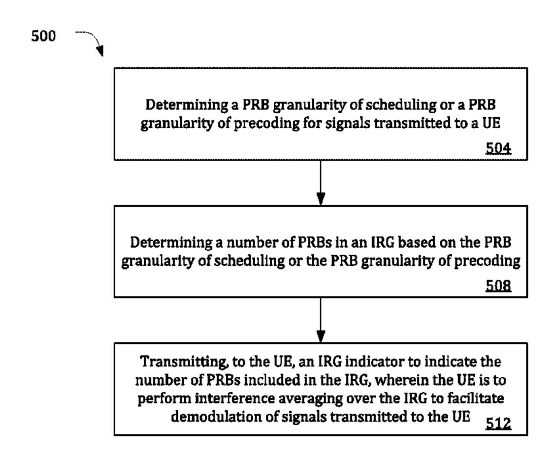
averaging interference measurements in a frequency domain. Additionally, or alternatively, the eNB may transmit an interference resource group (IRG) indicator to the UE to indicate an IRG over which the UE is to perform interference averaging to facilitate demodulation of signals received by the UE from the eNB.
