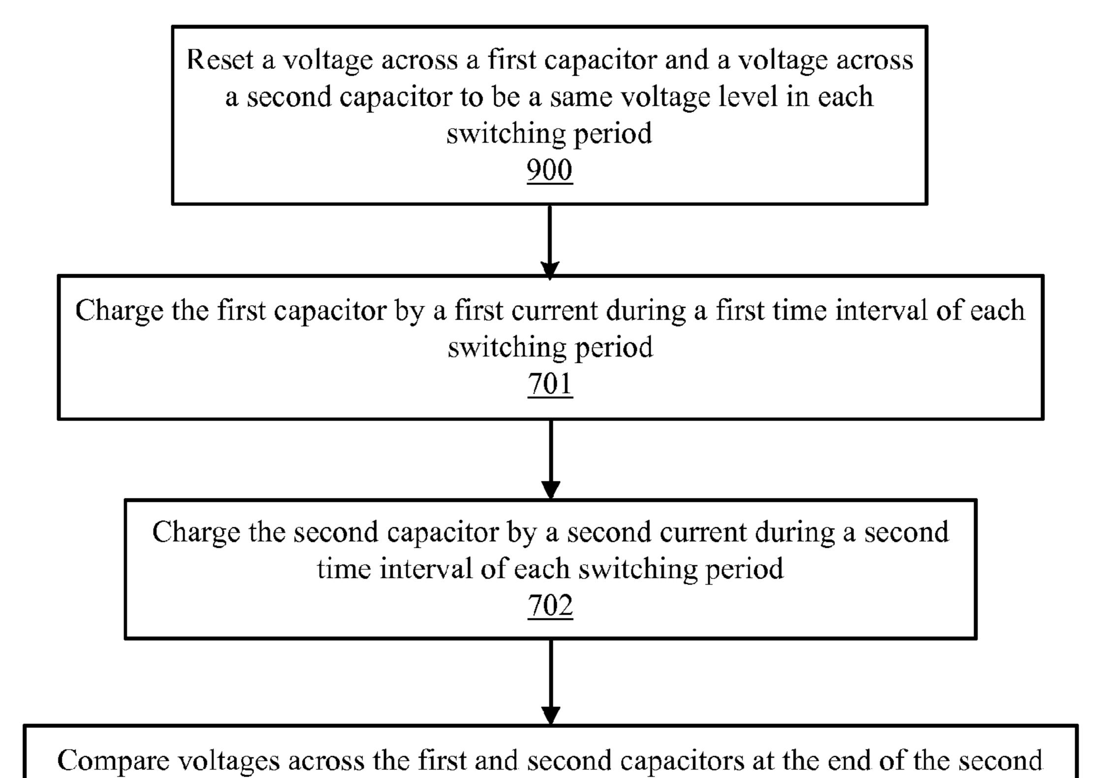
time interval to generate an overvoltage protection signal, where the overvoltage
