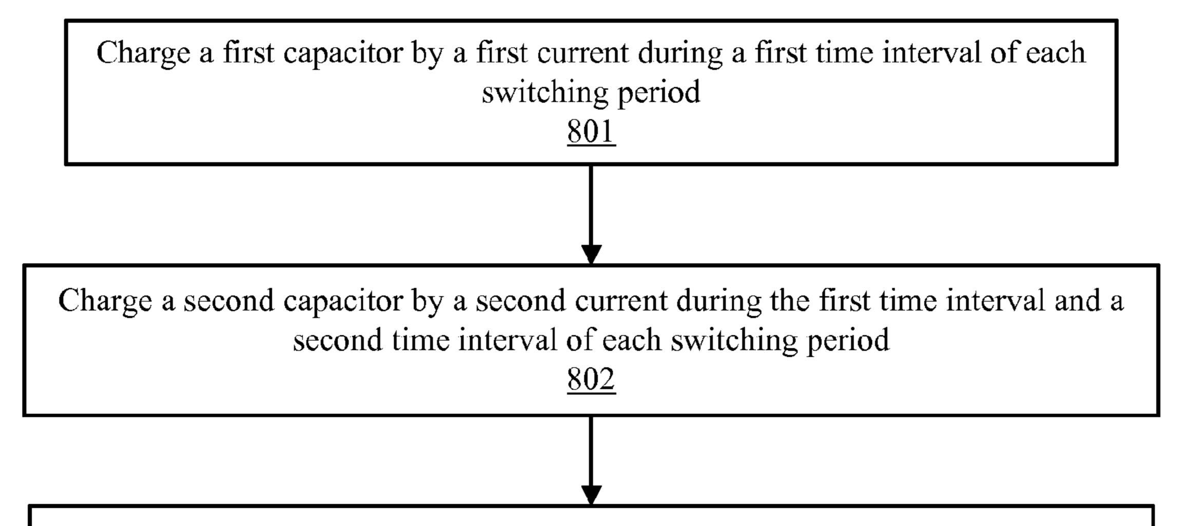
Compare voltages across the first and second capacitors at the end of second time interval to generate an overvoltage protection signal, where the overvoltage protection signal is active when voltage the voltage across the first capacitor is not less than the voltage across the second capacitor at the end of second time interval 803
