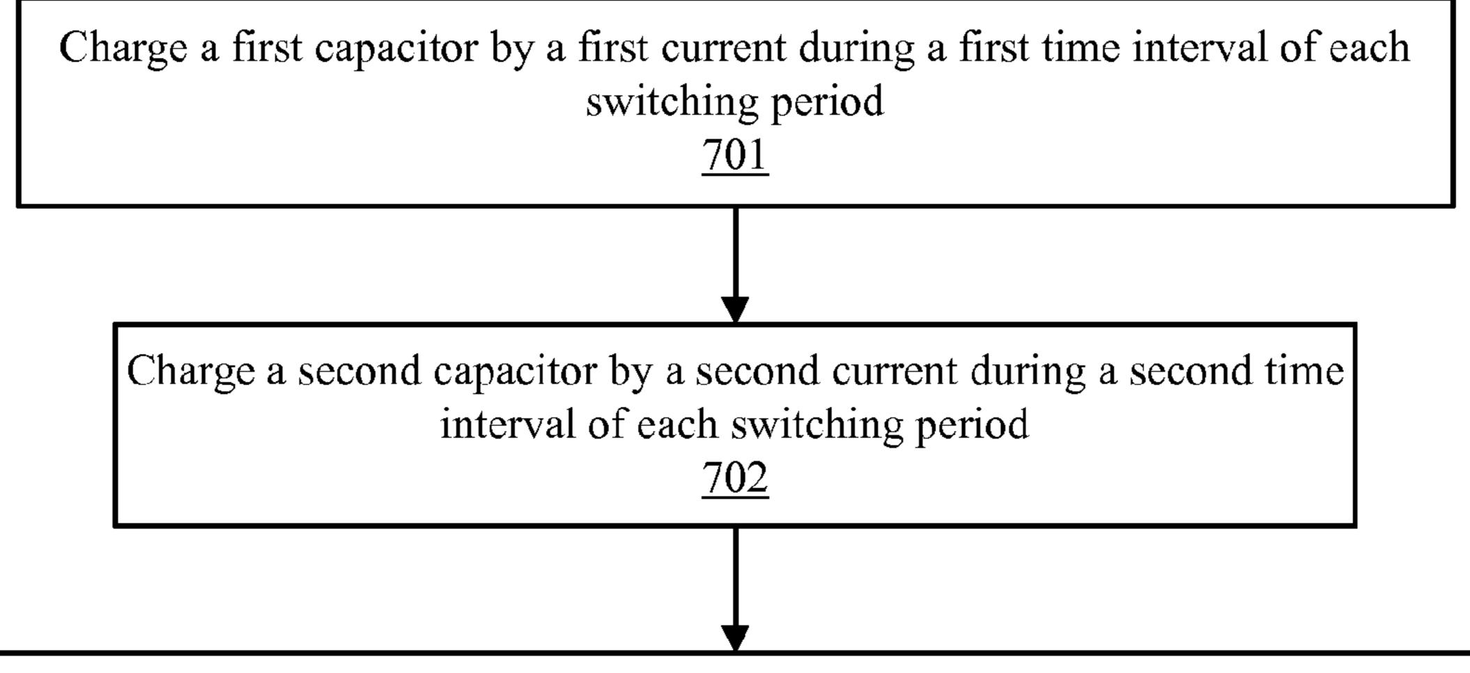
Compare voltages across the first and second capacitors at the end of the second time interval to generate an overvoltage protection signal, where the overvoltage protection signal is active when voltage across the first capacitor is not less than the voltage across the second capacitor at the end of second time interval
