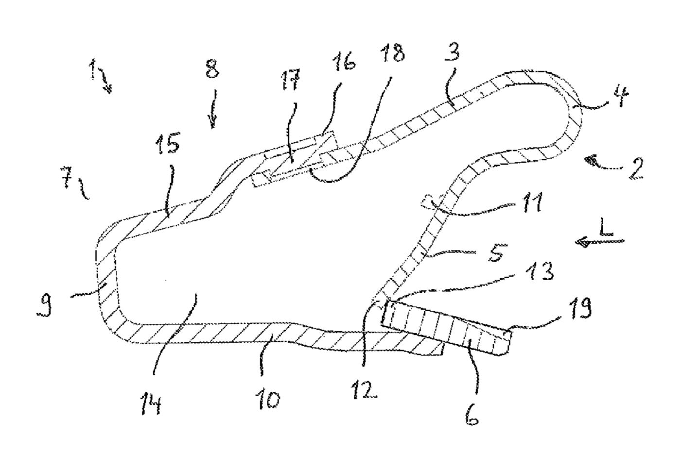
to be clamped, a conductor-accommodating space (14) for accommodating a free end of the electrical conductor. The base portion (10) extends from the curved portion (9) toward the free end of the base portion (10) counter to the insertion direction (L) of an electrical conductor to be clamped.
