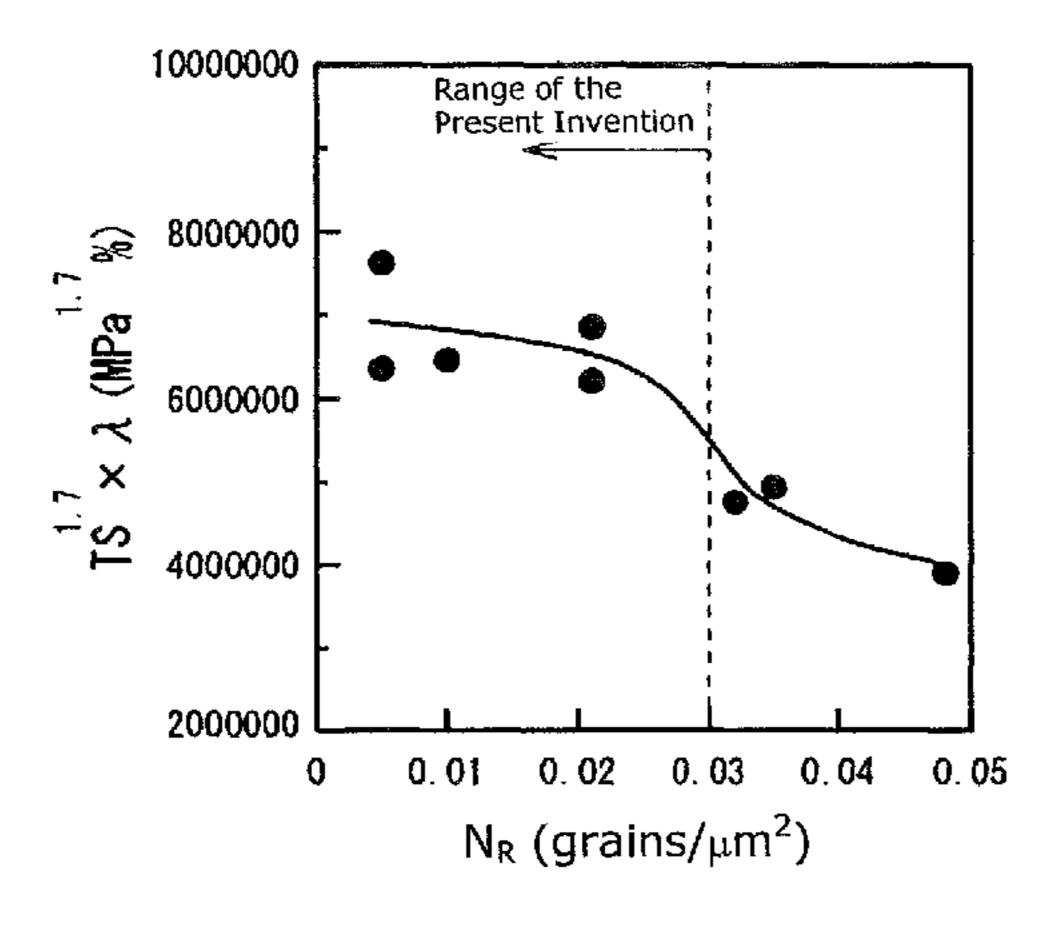
4.0% to less than 25.0% and an average grain size of less than 0.80  $\mu$ m, and of the retained austenite, the number density of retained austenite grains whose grain size is 1.2  $\mu$ m or more is  $3.0 \times 10^{-2}$  grains/ $\mu$ m<sup>2</sup> or less.
