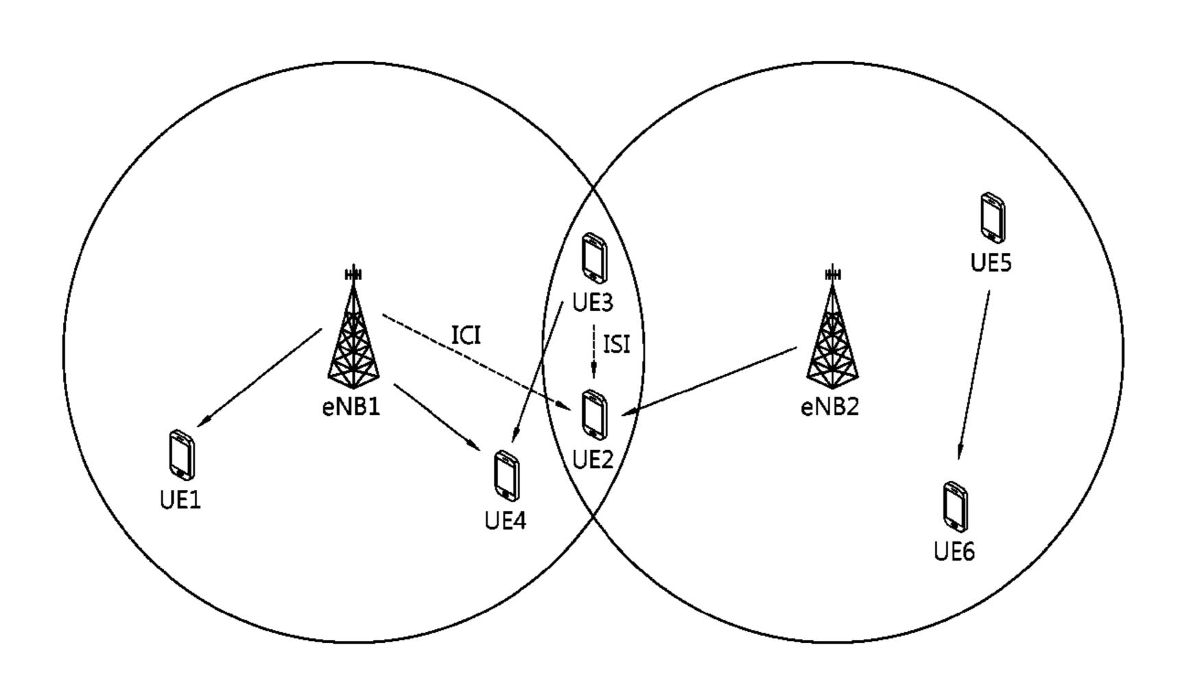
downlink control channel which is transmitted from a cellular base station to a cellular terminal. The control apparatus determines an interference candidate resource, which is subject to inter-cell interference control, on the basis of the downlink control channel. A step of the control apparatus transmitting an interference control message to a D2D terminal using the interference candidate resource is included.
