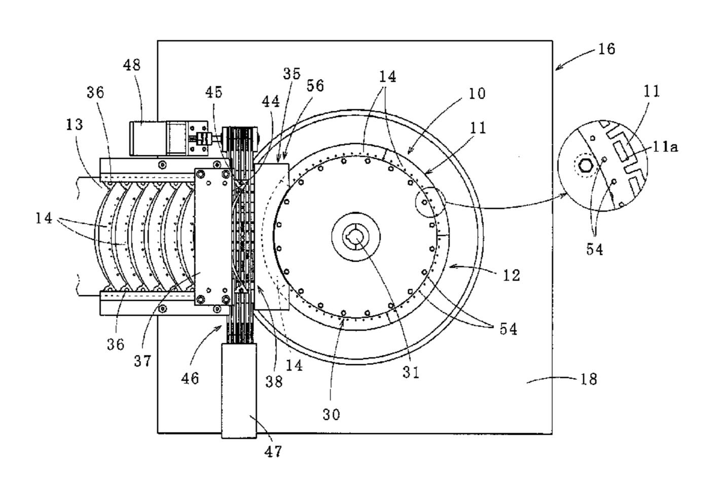
core piece therein is rotated by 360°/m and a second process that the first process is repeated to form an annularly connected iron core piece in which the segment iron core pieces are annularly arranged. The second process is repeated to form a caulked and laminated iron core having a prescribed thickness. During the second process, the segment iron core pieces are caulked and laminated in the rotary laminating mechanism.
