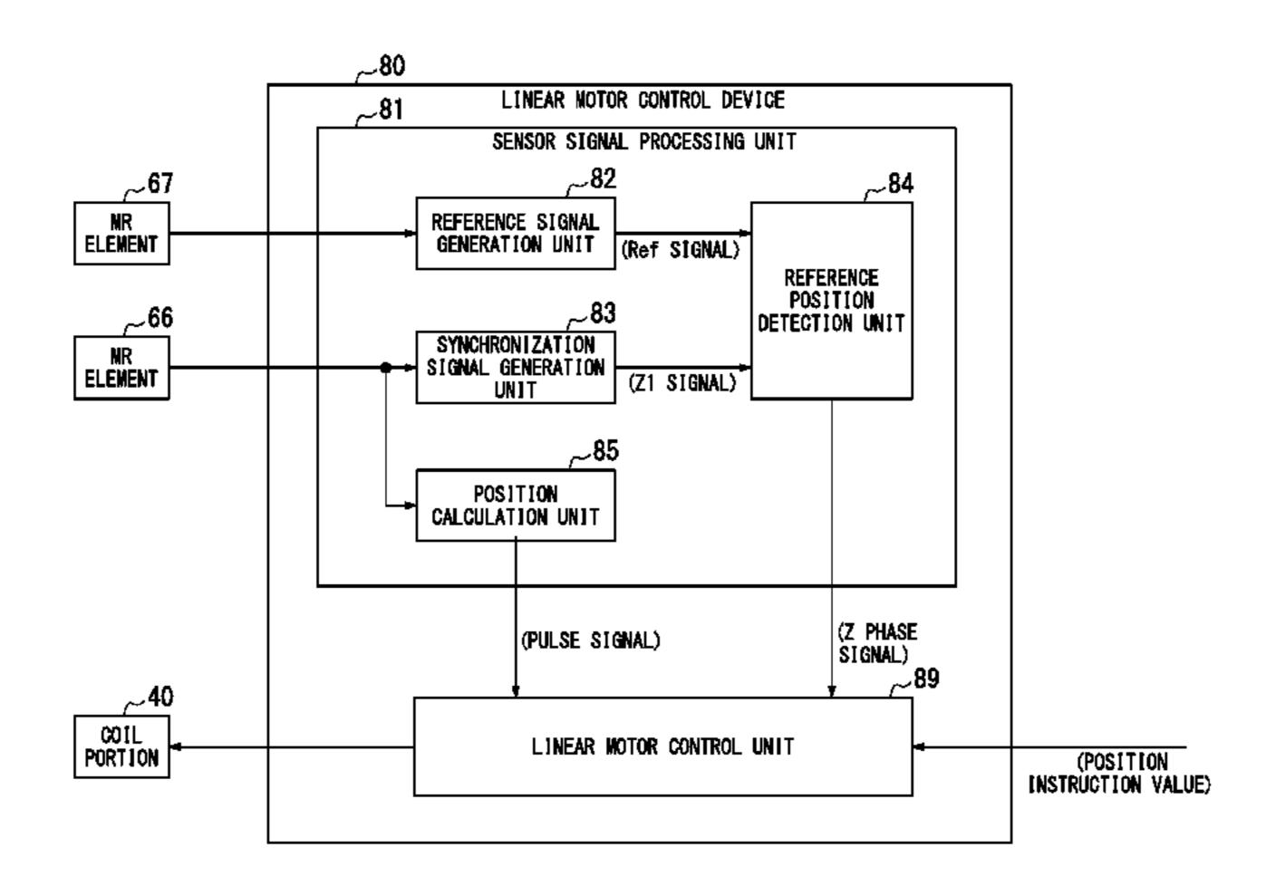
after the reference signal generation unit (82) generates the pulse signal.
