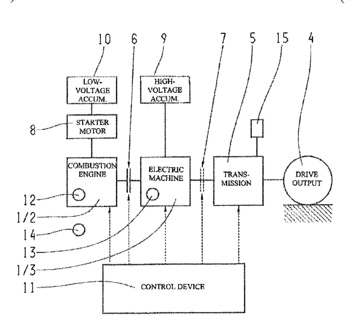
least the transmission and the clutch connected between the internal combustion engine and the electric machine of the hybrid drive unit to a condition appropriate for the starting mode determined by emitting appropriate control signals.
