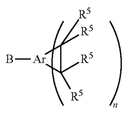
wherein B is an n-valent linking group; Ar is a polyvalent aryl group and the carbon atoms of the cyclobutene ring are bonded to adjacent carbon atoms on the same aromatic ring of Ar; n is an integer of 1 or more; and R<sup>5</sup> is a monovalent group.
