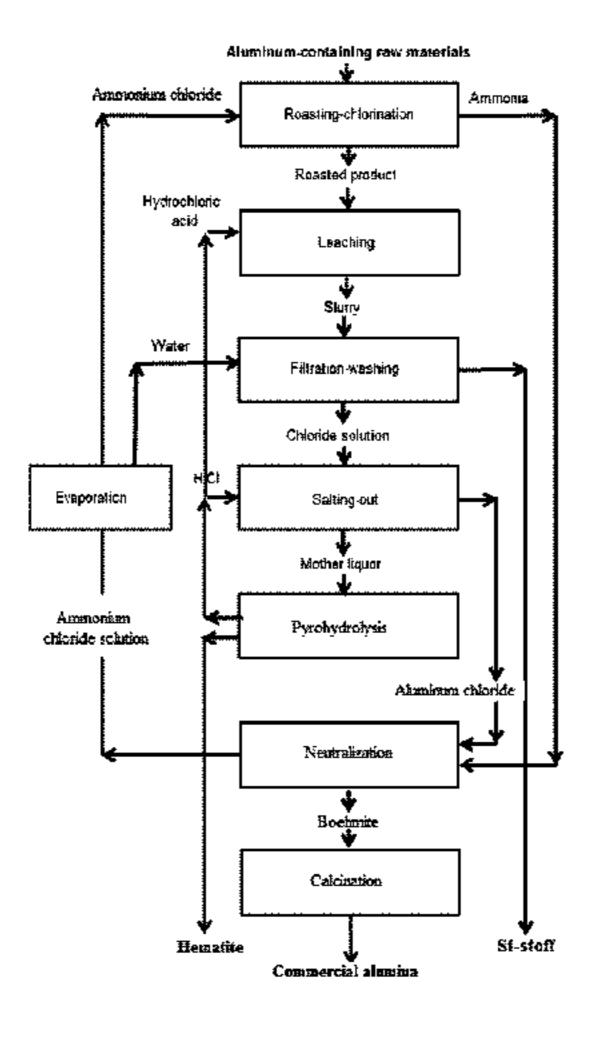
released during the evaporation can be mixed with the aluminum-containing raw material.
