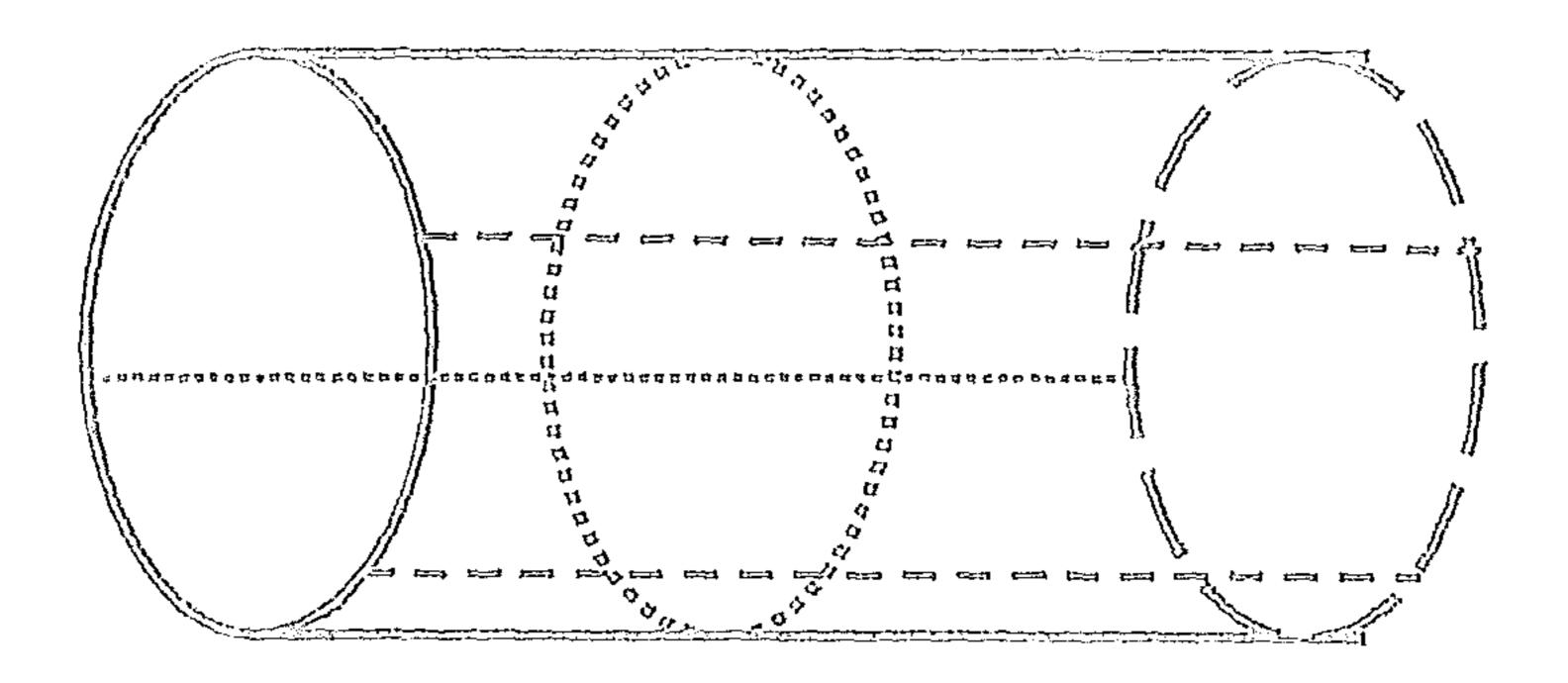
Figure 2. A plug wrap having 60 holes/inch
