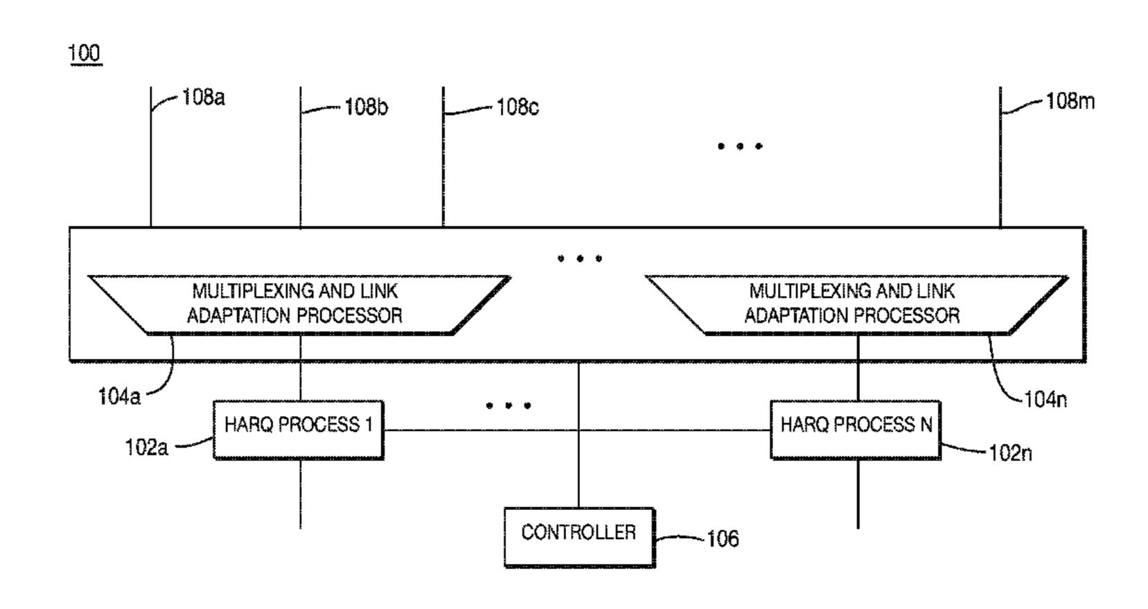
H-ARQ process are determined. TBs are generated from the mapped higher layer data in accordance with the physical transmission and H-ARQ configurations of each H-ARQ process, respectively. The TBs are transmitted via the H-ARQ processes simultaneously.
