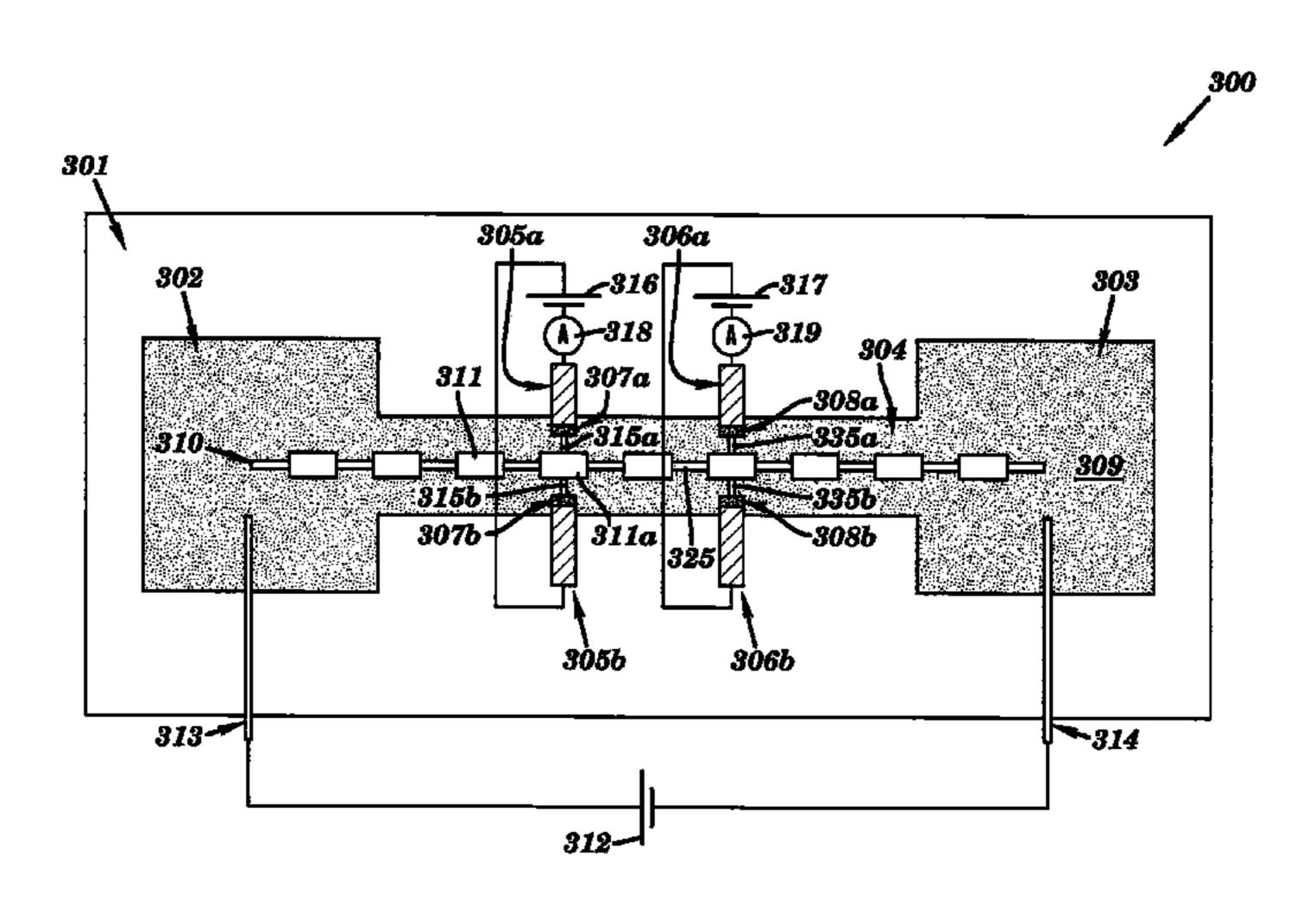
for motion control, and the second type forms first and second transient bonds to different bonding sites of a base of the molecule. When a voltage is applied to the pair of electrode layers a tunneling current is generated by the base in the nanopore, and the tunneling current travels via the first and second transient bonds formed to be measured as a current signature for distinguishing the base. The motion control transient bond is stronger than first and second transient bonds.
