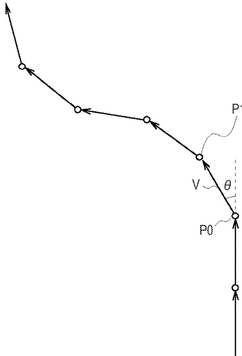
CURRENT POSITION CALCULATION METHOD USING VELOCITY AND ANGLE
