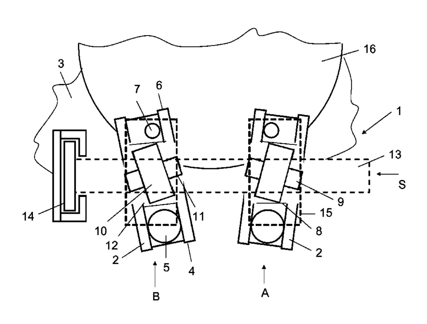
from perpendicular, and d) a partial quantity of the first and second main group (A, B) are selected and mounted for each row of cam followers (2) in order to minimize/compensate for an axial thrust of the camshaft (13).
