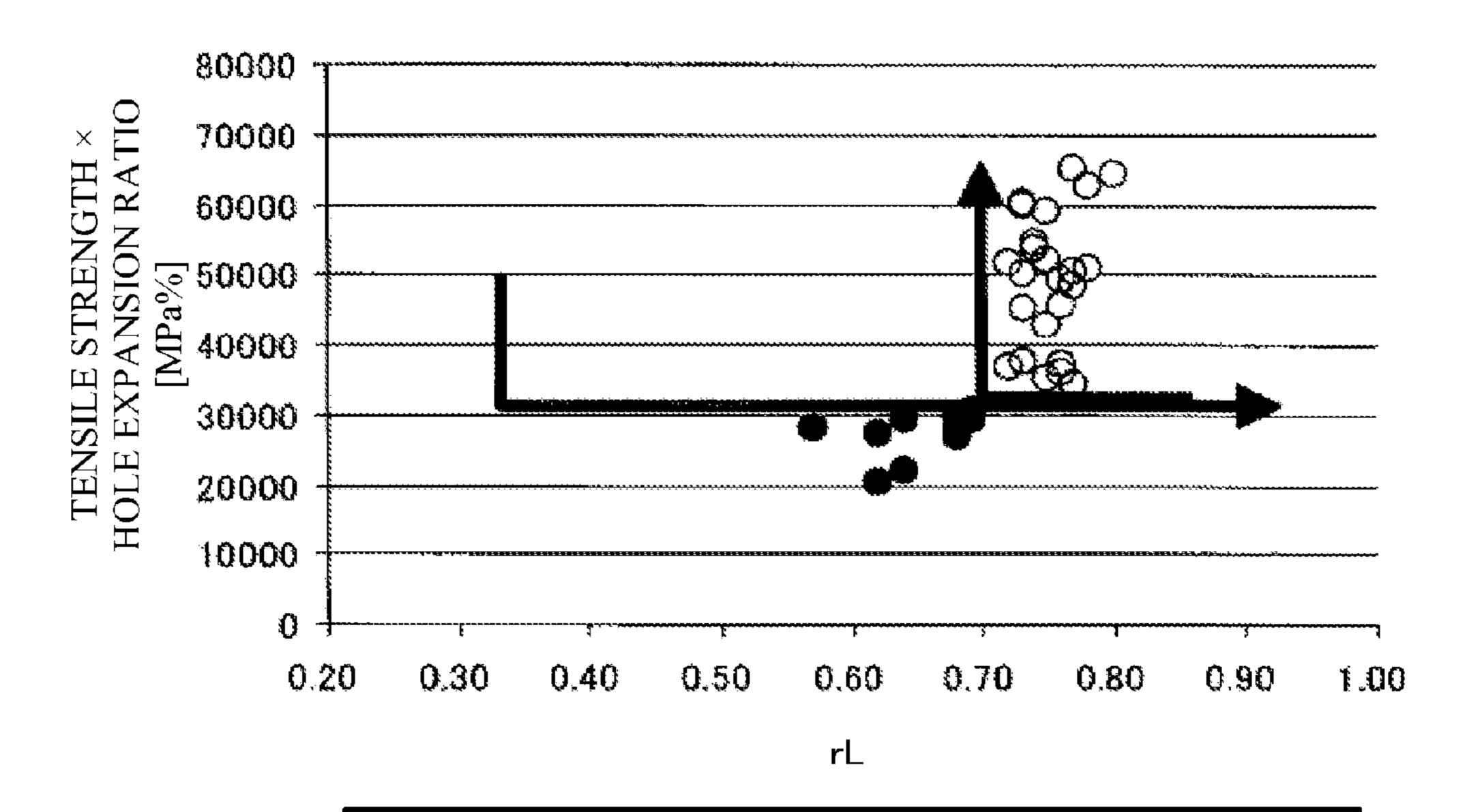
O: IN FIG. 1 AND FIG. 2, POLE DENSITIES OF TWO TYPES OF ORIENTATION GROUPS ARE WITHIN RANGE OF CLAIMS AND  $rL \ge 0.70$
