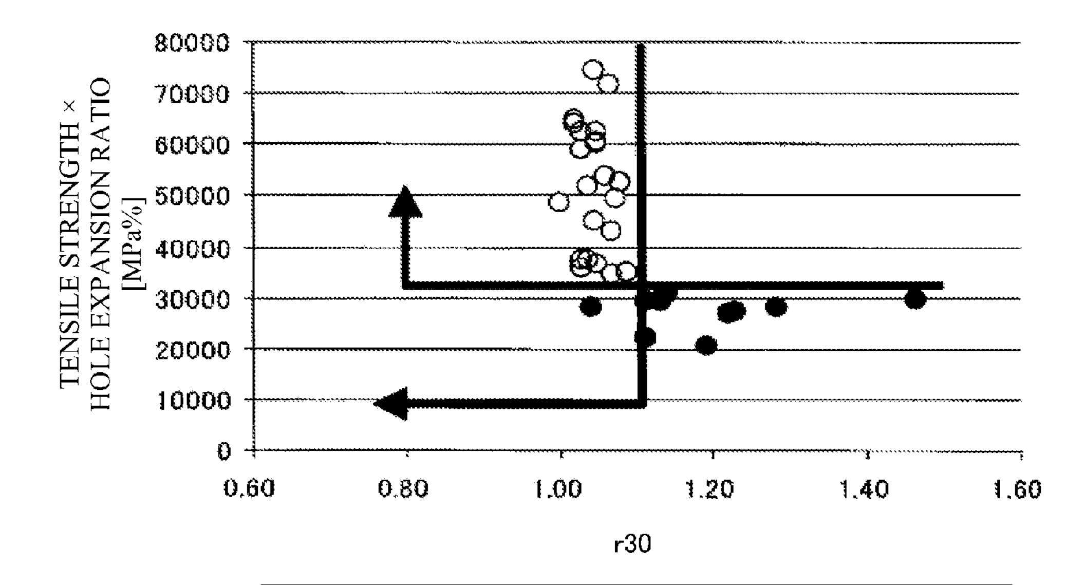
O: IN FIG. 1 AND FIG. 2, POLE DENSITIES OF TWO TYPES OF ORIENTATION GROUPS ARE WITHIN RANGE OF CLAIMS AND  $r30 \le 1.10$
