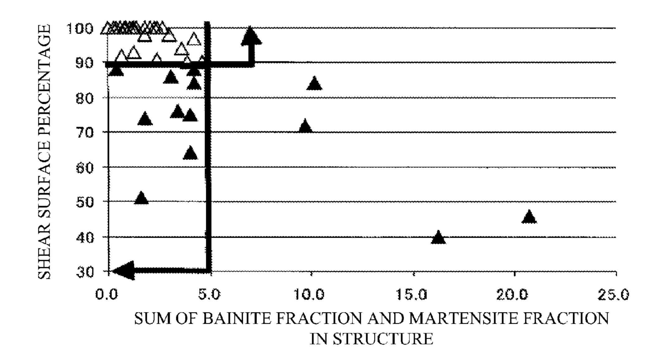
O: IN FIG. 1 AND FIG. 2, POLE DENSITIES OF TWO TYPES OF ORIENTATION GROUPS ARE WITHIN RANGE OF CLAIMS AND SHEAR SURFACE PERCENTAGE ≥ 90%
