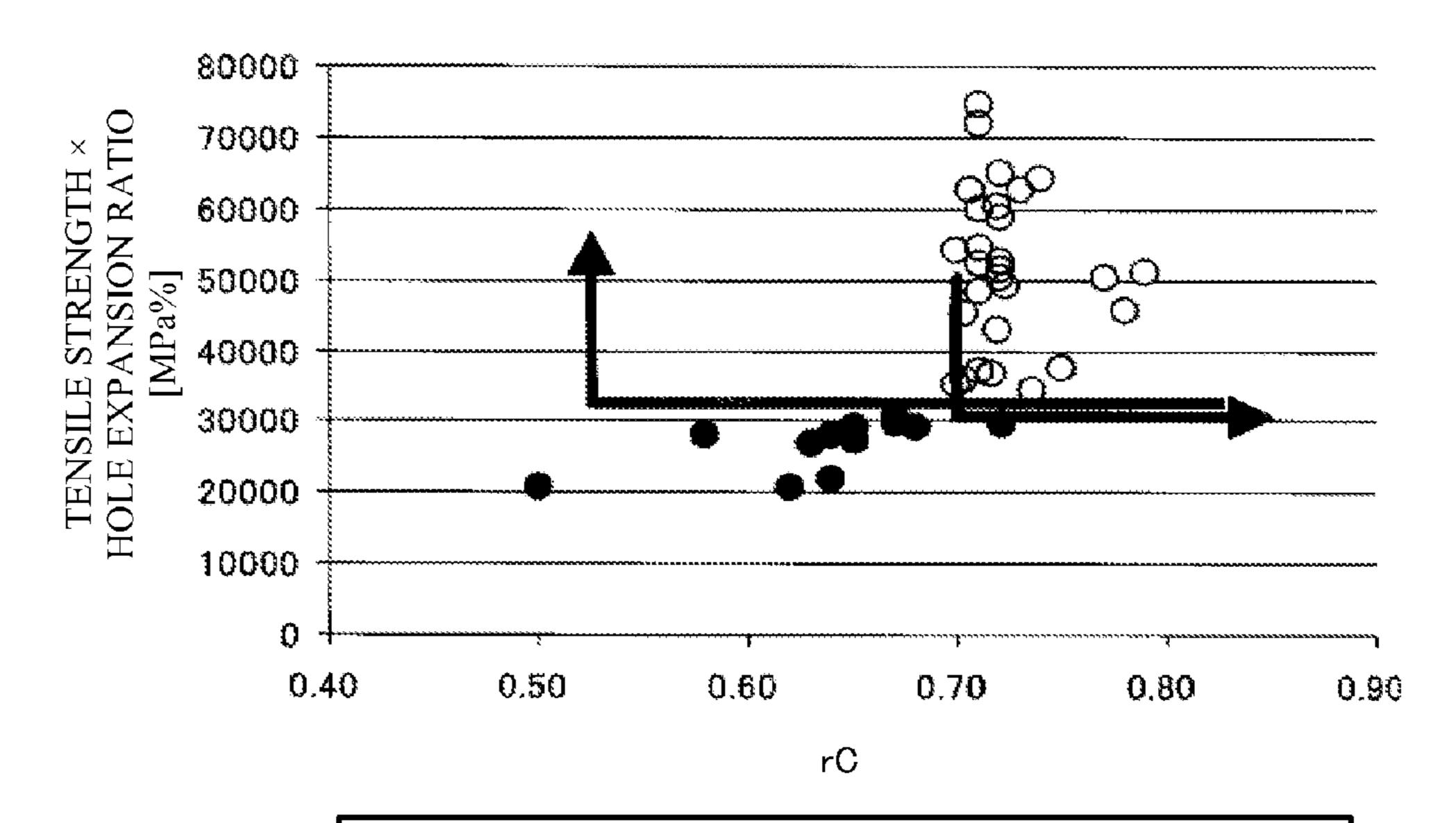
O: IN FIG. 1 AND FIG. 2, POLE DENSITIES OF TWO TYPES OF ORIENTATION GROUPS ARE WITHIN RANGE OF CLAIMS AND  $rC \ge 0.70$
