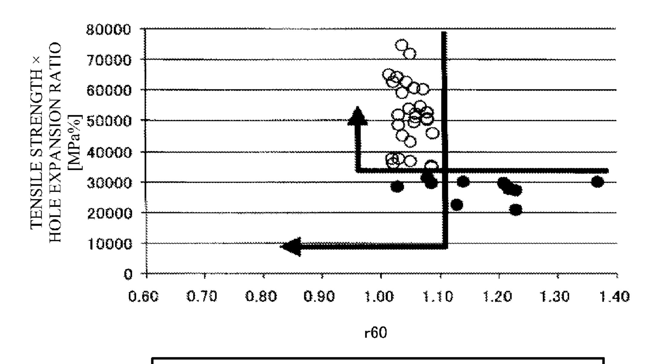
O: IN FIG. 1 AND FIG. 2, POLE DENSITIES OF TWO TYPES OF ORIENTATION GROUPS ARE WITHIN RANGE OF CLAIMS AND  $r60 \le 1.10$
