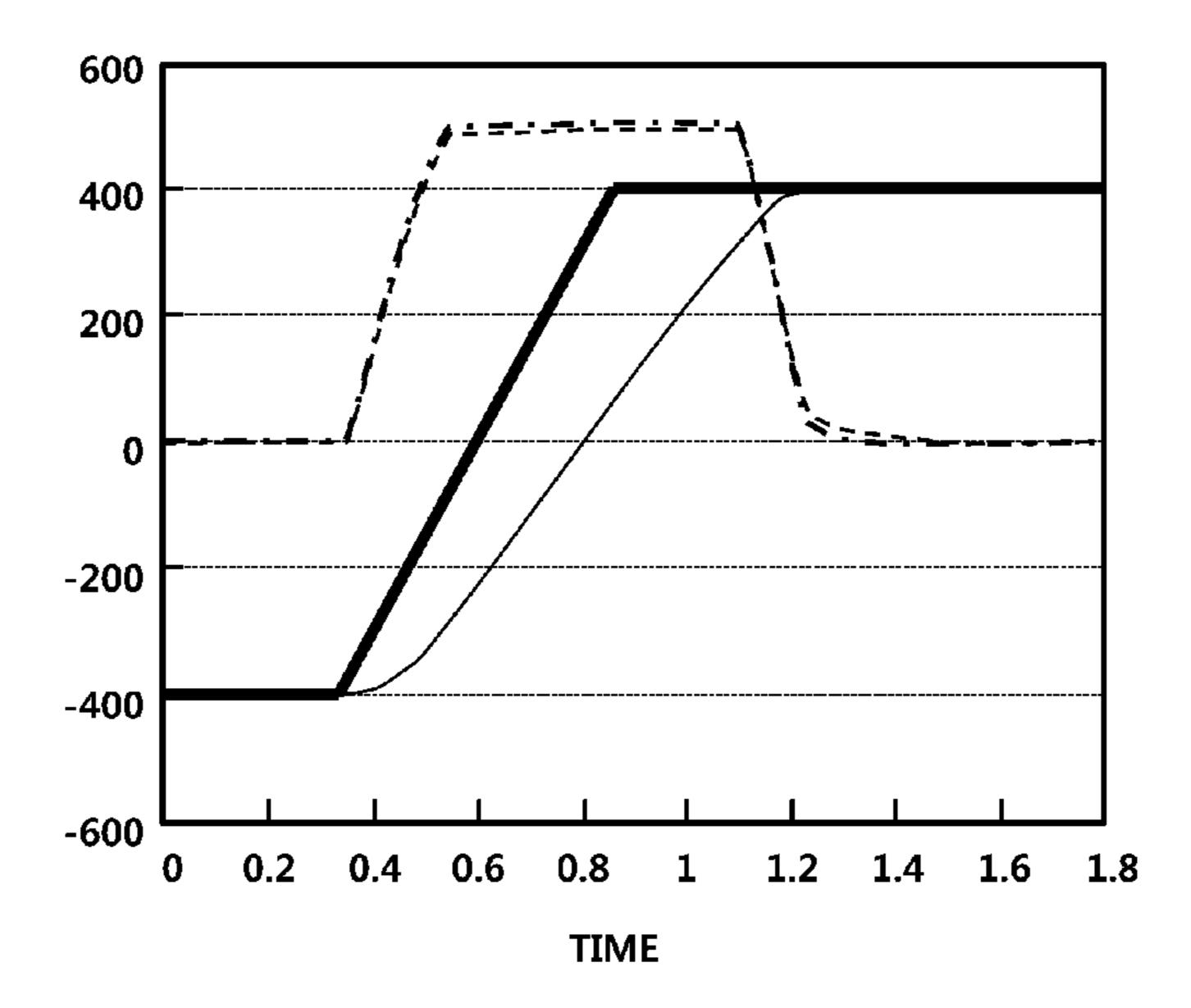
TARGET MOTOR ROTATION ANGLE **MOTOR ROTATION ANGLE** TARGET MOTOR ANGULAR VELOCITY **MOTOR ANGULAR VELOCITY**
