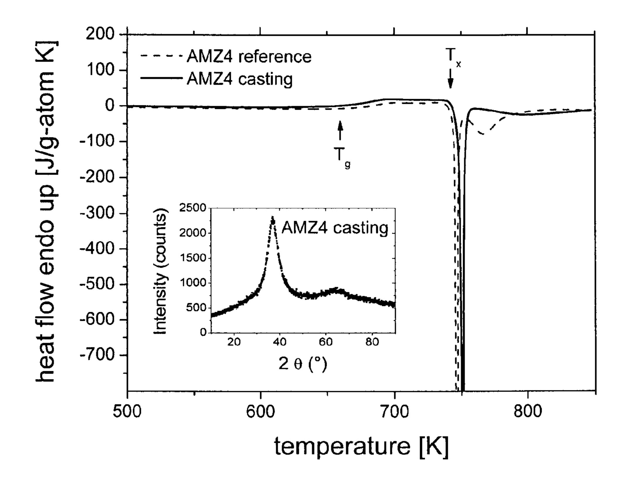
AMZ4 =  $yL_{com}$  xCu zAl wherein x = 71.9 wt%, y = 24.4 wt%, and z = 3.7 wt%
