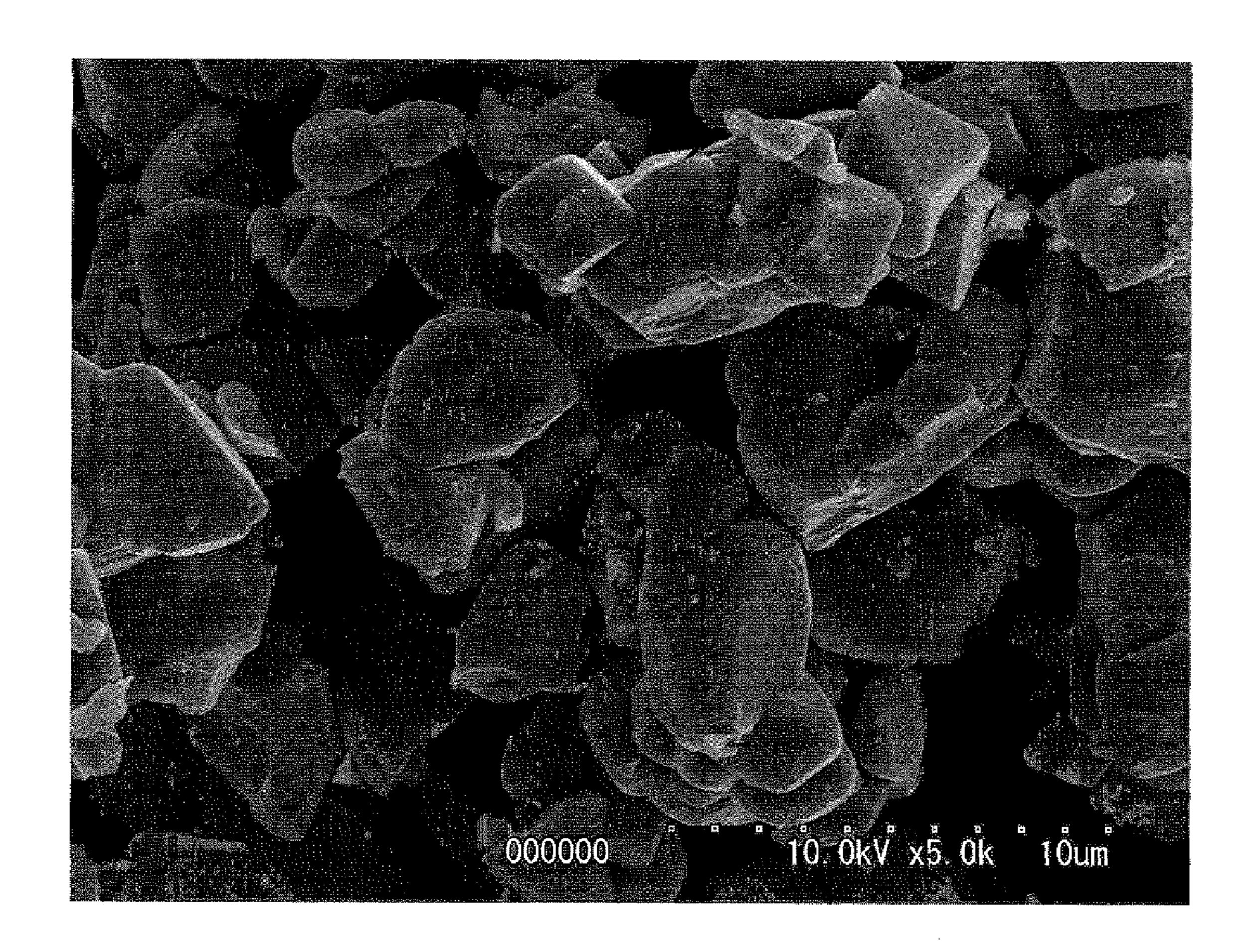
POSITIVE ELECTRODE ACTIVE MATERIAL FOR SECONDARY BATTERIES WITH NONAQUEOUS ELECTROLYTIC SOLUTION, PROCESS FOR THE PRODUCTION OF THE ACTIVE MATERIAL, AND SECONDARY BATTERIES WITH NONAQUEOUS ELECTROLYTIC SOLUTION
